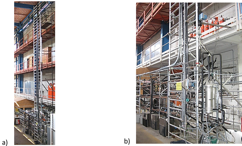
Figure 2. 2: Archimède flowloop in the SPIN laboratory: (a) vertical section and (b) horizontal section.
