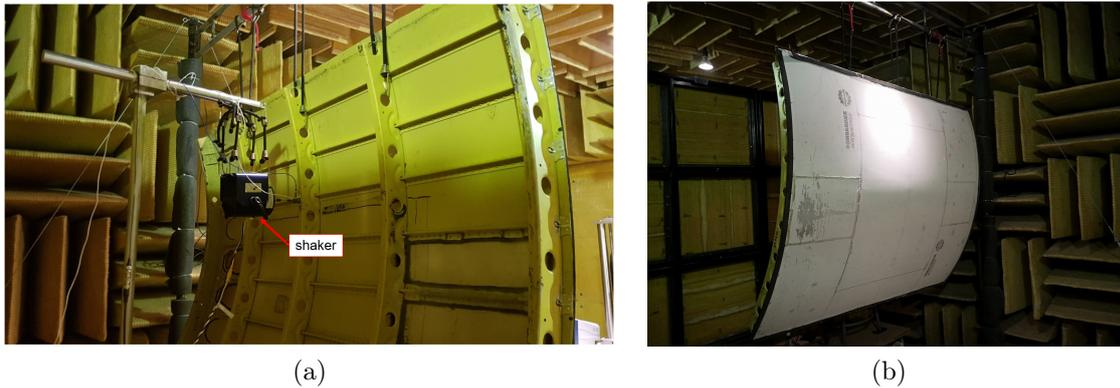
Figure 4.7 – Set-up and installation for mechanical excitation: shaker installation (a) and acquisition region (b).
