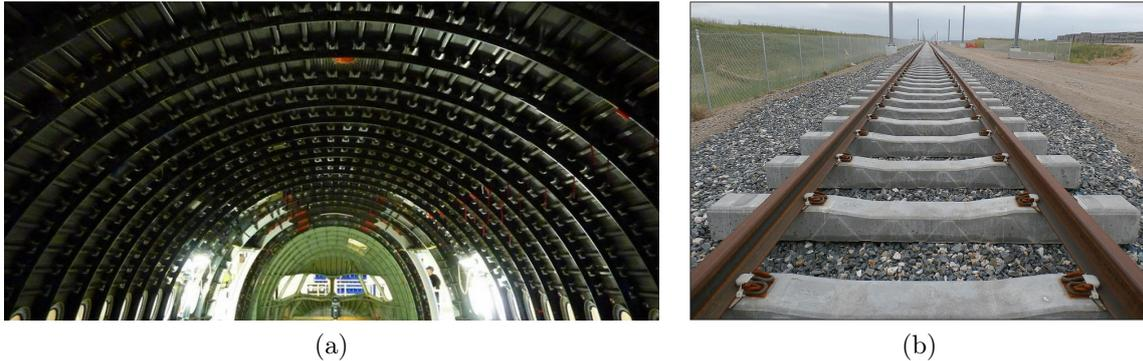
Figure 0.2 – Periodic structures: part of the fuselage of an AIRBUS A350 aircraft (a) and a rail (b).
