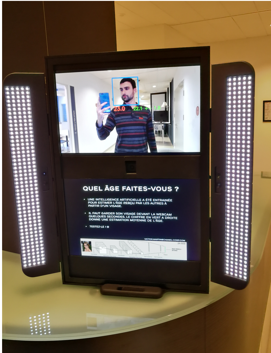
Figure A.1 – The color and the brightness of the lights are controlled by the mirror. The red number is the instant estimate and the two green numbers are the mean and standard deviation over the 40 last estimates.
