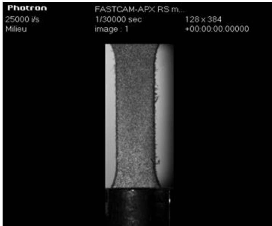
Figure 4-2 First image at undeformed stage of dynamic PP tensile specimen (global size of 512x472 pixels vs. useful part of 128x384 pixels).
