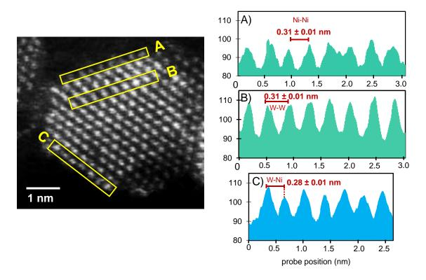
**Figure 50.** Variations of contrast and interatomic distances at different zones of a sulfided slab of NiW (CA/Mo=2)/Al<sub>2</sub>O<sub>3</sub> (particle with right with dotted frame in Figure 9C).
