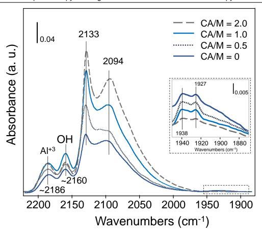
**Figure 43.** IR spectra of CO adsorption (133 Pa CO at equilibrium, T<sub>ads</sub>=100K) on NiW(CA/M=x)/Al<sub>2</sub>O<sub>3</sub> catalysts sulfided at 673K. The inset zooms on the low wavenumber bands.
