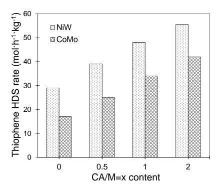
**Figure 42.** Effect CA addition on thiophene HDS activity of sulfided NiW(CA/M=x)/Al<sub>2</sub>O<sub>3</sub> catalysts sulfided at 673 K and CoMo(CA/M=x)/Al<sub>2</sub>O<sub>3</sub> catalysts sulfided at 623 K.
