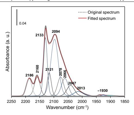
**Figure 46.** Decomposition of the IR spectrum of CO adsorption (PCO=133 Pa at equilibrium, T=100 K) on NiW(CA)/Al<sub>2</sub>O<sub>3</sub> catalyst sulfided at 673 K with Peakfit V4.12.
