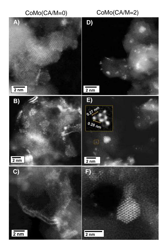
**Figure 54.** HR STEM-HAADF micrographs of CoMoS particles of CoMo(CA/M=0)/ Al<sub>2</sub>O<sub>3</sub> (A-C) and CoMo(CA/M=2)/Al<sub>2</sub>O<sub>3</sub> (D-F) of different zones. Inset E: zoom of particle with dispersion degree of 1.0.
