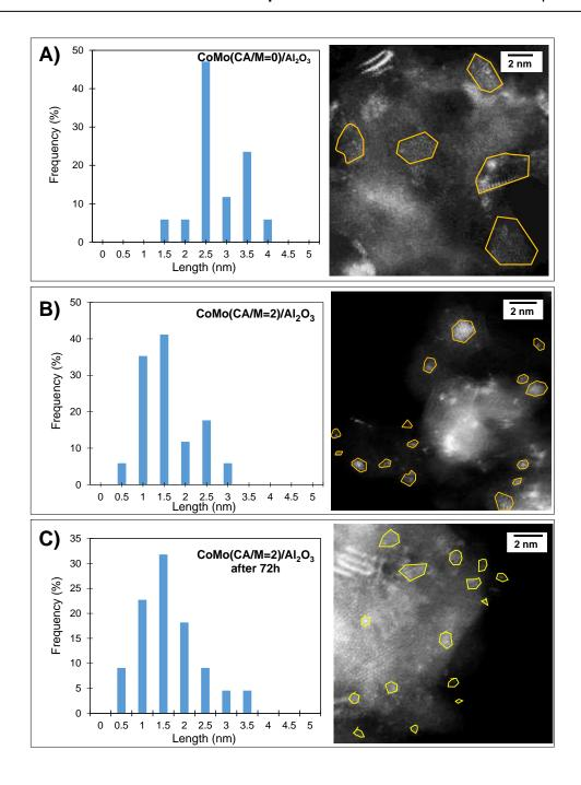
Moreover, by analyzing contrast and measurement of interatomic distances on HR STEM HAADF images of sulfide particles, it was possible to identify the nature of the core and edge atoms of the W- and Mo-based particles. On both systems, it appears the edges of the particles could be either fully promoted with detection of only Ni or Co, or partially promoted with detection of both Ni
