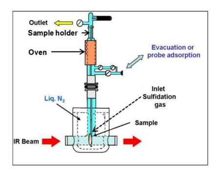
Figure 25. IR cell at low temperature
