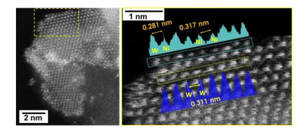
**Figure 51.** HR HAADF-STEM image of sulfided NiW(CA/M=2)/Al<sub>2</sub>O<sub>3</sub> catalyst. Inset of the figure shows the contrast variations and characteristic distances observed in the atoms located in the periphery and in the bulk of the slab.
