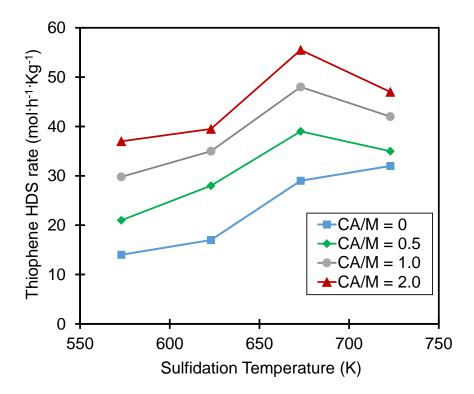
**Figure 41.** Effect of sulfidation temperature of NiW(CA/M=x)/Al<sub>2</sub>O<sub>3</sub> catalysts on the thiophene HDS activity.
