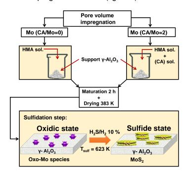
**Figure 1.** Scheme of preparation of sulfide conventional Mo catalysts for HDS.
