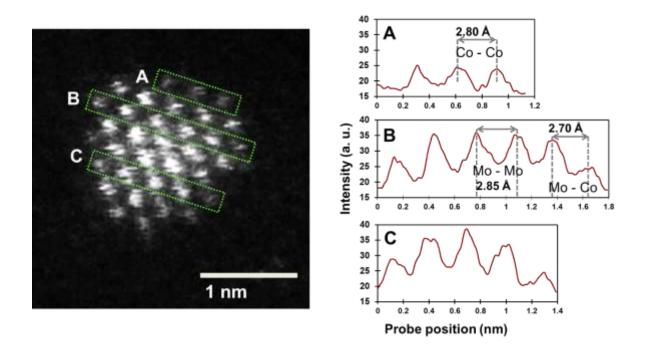
**Figure 57.** STEM-HADDF image of sulfided CoMo(CA/M=2)/Al<sub>2</sub>O<sub>3</sub> with the corresponding intensity profiles measured at different regions of the slab. The spacing between the Co-Co, Mo-Mo and Co-Mo was revealed by this profile.
