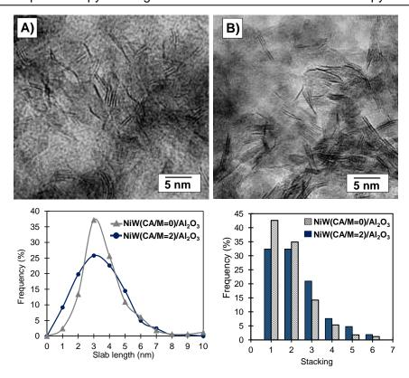
**Figure 48**. HRTEM images of NiW(CA/M=0)/Al<sub>2</sub>O<sub>3</sub> (A) and NiW(CA/M=2)/Al<sub>2</sub>O<sub>3</sub> (B), with their slab length distribution and stacking number distribution.
