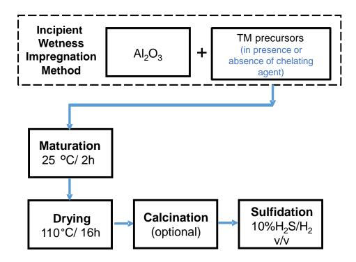
**Figure 4.** Scheme of preparation of sulfide conventional catalysts for HDS.
