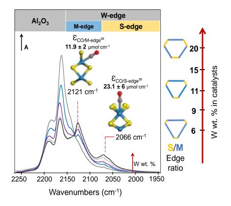
The integrated molar attenuation coefficients of CO associated with the M-and S-edge sites were successfully determined, allowing determination of the WS<sub>2</sub> morphology. Increasing the W loading (3-20 wt% W) allows going from an almost pure triangle exhibiting mostly M-edge to a truncated hexagon.
