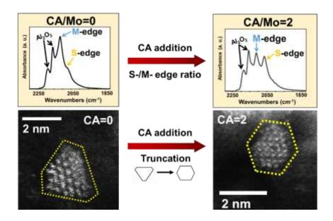
As a consequence, this study strengthens the importance of coupling techniques like microscopy that allows a direct observation of the shape of a group of sulfided slabs and IR spectroscopy that allows an indirect detection of the shape but of a large number of sulfided slabs.
