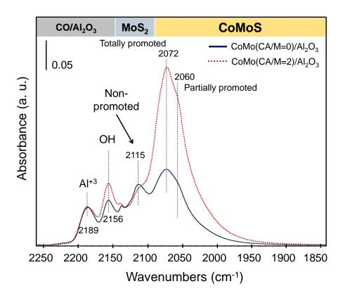
**Figure 52.** IR spectra of CO adsorption (-173 °C and 133 Pa CO at equilibrium) on CoMo(CA/M=0)/Al<sub>2</sub>O<sub>3</sub> and CoMo(CA/M=2)/Al<sub>2</sub>O<sub>3</sub> catalysts sulfided with 10% (v/v) H<sub>2</sub>S/H<sub>2</sub> at atmospheric pressure and 350 °C for 2 h.
