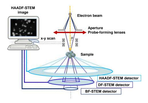
Figure 28. Representative example of the STEM system.
