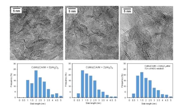
**Figure 53.** HRTEM analysis of slab length distribution: images of CoMo(CA/M=0)/Al2O3, CoMo(CA/M=2)/Al<sub>2</sub>O<sub>3</sub> and CoMo(CA/M=2)/ Al<sub>2</sub>O<sub>3</sub> after 72 h of thiophene reaction.
