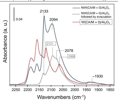
**Figure 44.** IR spectra of CO adsorbed on sulfided NiW(CA/M=0)/Al<sub>2</sub>O<sub>3</sub> and W(CA/M=0)/Al<sub>2</sub>O<sub>3</sub>. Continuous lines: spectra taken at 100K in presence of  $P_{equil} = 133$  Pa CO. Dotted line: spectra taken after evacuation of CO at room temperature until reaching P<1  $10^{-4}$  Pa.
