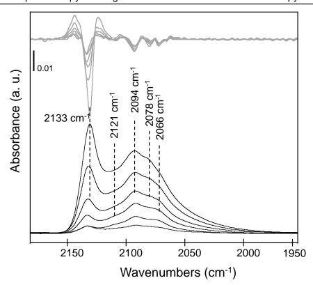
Figure 45. IR spectra of first CO doses (0.002 to 0.012  $\mu$ mol CO·mg<sup>-1</sup>) adsorbed at 100 K on NiW(CA/M=0)/Al<sub>2</sub>O<sub>3</sub> sulfided at 673 K. Each spectrum is presented with its second derivative function (lighter curves).
