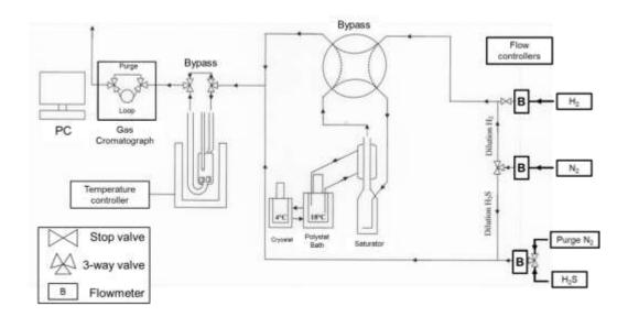
Figure 29. Thiophene test set up
