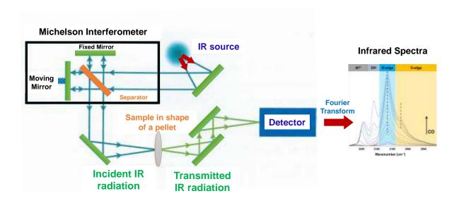
**Figure 22.** Scheme of the principle of functioning of an IR spectrometer.
