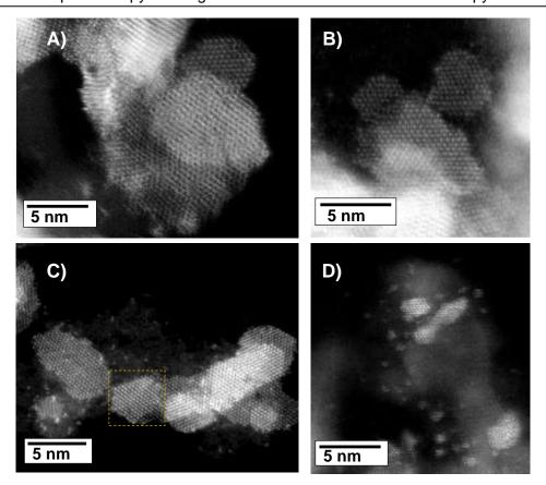
**Figure 49**. HR STEM-HAADF micrographs of NiWS particles of NiW(CA/M=0)/Al<sub>2</sub>O<sub>3</sub> (A and B) and NiW(CA/M=2)/Al<sub>2</sub>O<sub>3</sub> (C and D).
