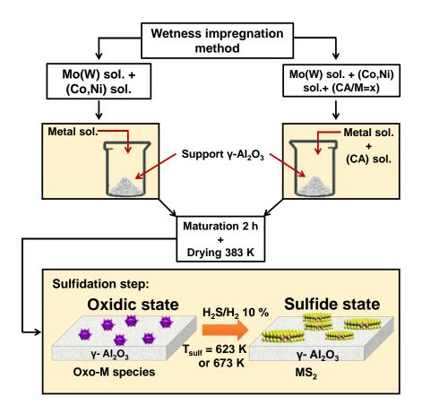
**Figure 20.** Catalyst preparation scheme used for the materials studied in this thesis.
