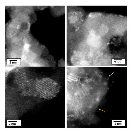
Figure 55. HR STEM-HAADF micrographs of CoMoS particles of CoMo(CA/M=2)/Al<sub>2</sub>O<sub>3</sub> after 72 h of thiophene HDS reaction at 623K. The arrows indicate that the few atoms agglomerates observed in CoMo(CA/M=2)/Al<sub>2</sub>O<sub>3</sub> after sulfidation are still present.
