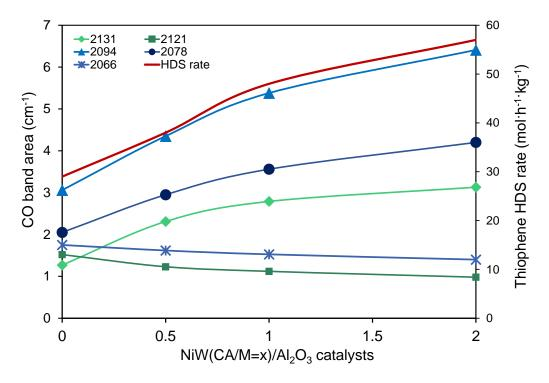
**Figure 47.** Effect of citric acid addition on the areas of different bands of the sulfided NiW (CA/M=x)/Al<sub>2</sub>O<sub>3</sub> catalysts obtained by CO/IR. In this graphic the HDS thiophene rate divided by a factor of ten is presented to evidence the parallel growth of certain bands along with the catalytic activity.
