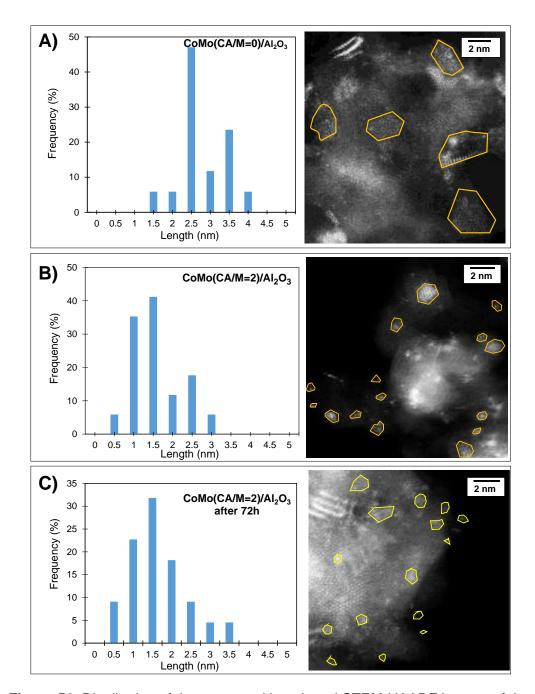
**Figure 56.** Distribution of the measured length and STEM-HAADF images of the particles of CoMo(CA/M=0)/Al<sub>2</sub>O<sub>3</sub>, CoMo(CA/M=2)/Al<sub>2</sub>O<sub>3</sub> and CoMo(CA/M=2)/Al<sub>2</sub>O<sub>3</sub> after thiophene HDS reaction (72h).
