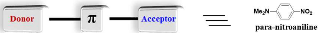
Figure 23. Schematic representation of a push-pull molecule composed of an EDG, a \pi -conjugated system and an EWG.
