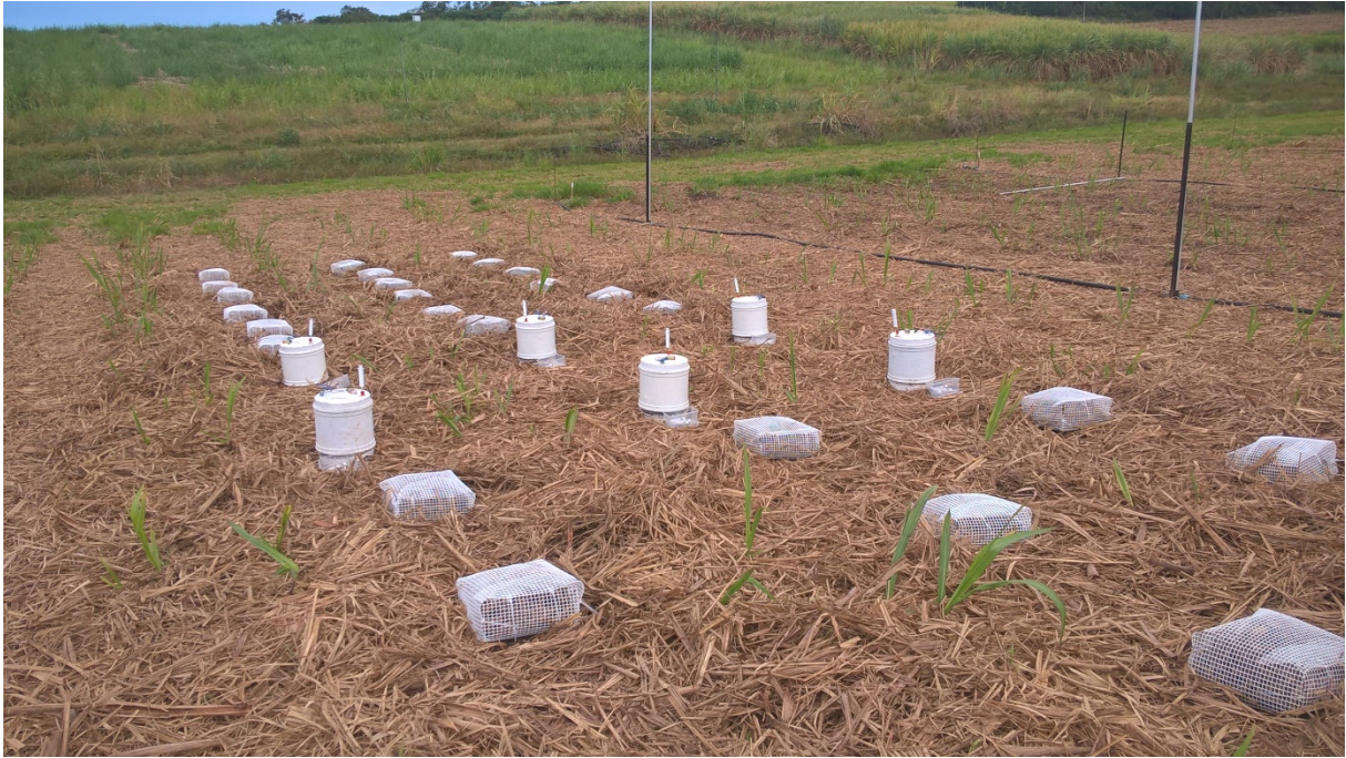
Figure 1: Design of litterbag and cylindrical chamber on-field experiments. Litterbags were used for measuring the decomposition of mulch or mulch-fertilizers mixtures, while cylindrical chambers were used for measuring CO 2 and N 2 O emissions from mulch or mulch-fertilizers mixtures. View of the plot with control treatments, with two quantities of sugarcane mulch, and 3 replicates.
