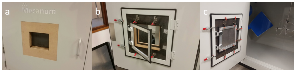
Figure 6.5: Facility and frame details: a) wooden external adaptive frame; b) clamping system on the internal chamber side; c) view of the open room with reflective panels and microphones.
