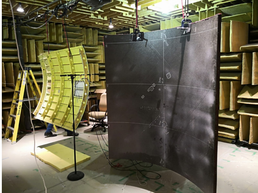
Figure 4.22: A view of the two test panels hanged in the the semi-anechoic chamber.
