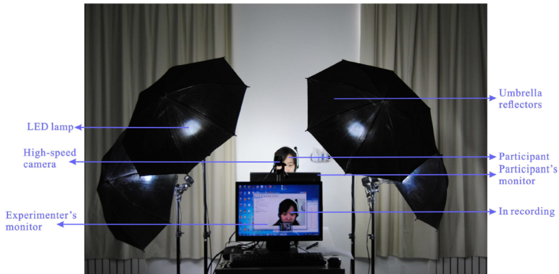
Figure 2-4: Acquisition setup for elicitation and recording of micro-expressions [135]
