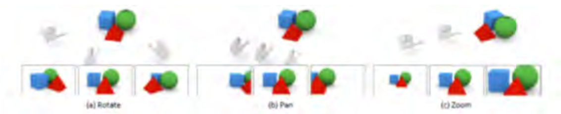
FIGURE 6 – Rotating, panning, and zooming are the primary camera movements used in almost every 3D modelling environments
