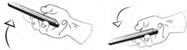
FIGURE 71 – DZ using gestural interactions via Accelerometer. Left : tilting the Smartphone towards the user’s body, Right : tilting the Smartphone faraway the user’s body
