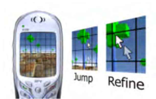
FIGURE 46 – Jump and Refine interaction technique
