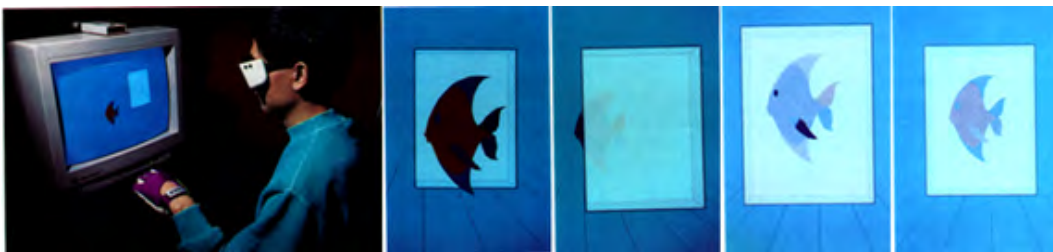
FIGURE 13 – Selecting a fish by using the Silk Cursor Technique (from left to right : The Silk Cursor Technique, A fish in front of the cursor, a fish behind the cursor, a fish partially inside the cursor, a fish completely inside the cursor)
