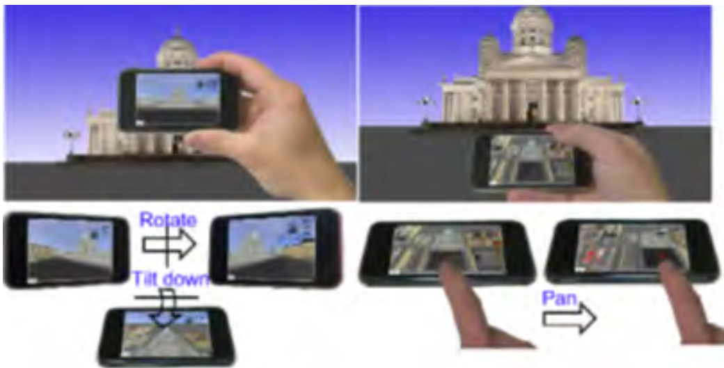
FIGURE 39 – POI interaction technique : left) the viewport is updated according to turning/rotation, and switched to the top-down view if turned to horizontal orientation, right) the user is operating the exocentric view by panning.
