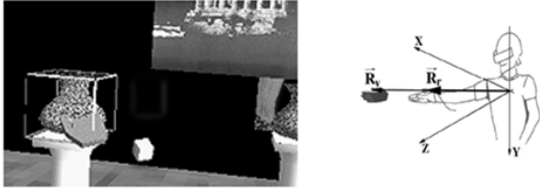
FIGURE 18 – Left : The Go-Go Technique, Right : The vector R_r represents the real hand position and the vector R_v represents the virtual hand position
