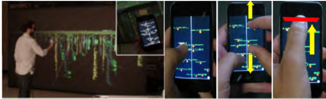
FIGURE 55 – The HandyMap interaction Technique. Left : the user points the target using a ray in a 3D VE, right : the subset of pointed objects is displayed on the iPod screen ; the refinement phase is applied via the touchscreen based interactions
