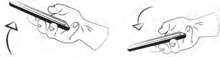
FIGURE 71 – DZ using gestural interactions via Accelerometer. Left : tilting the Smartphone towards the user’s body, Right : tilting the Smartphone faraway the user’s body
