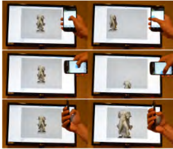
FIGURE 57 – Using the smartphone as a generic remote 3D interaction device
