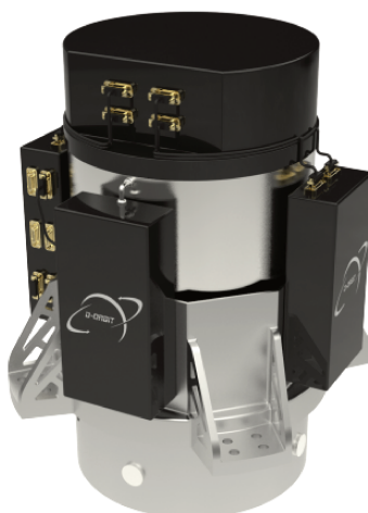
Figure II.6: D3 Decommissioning device. Credit: D-Orbit [84].
