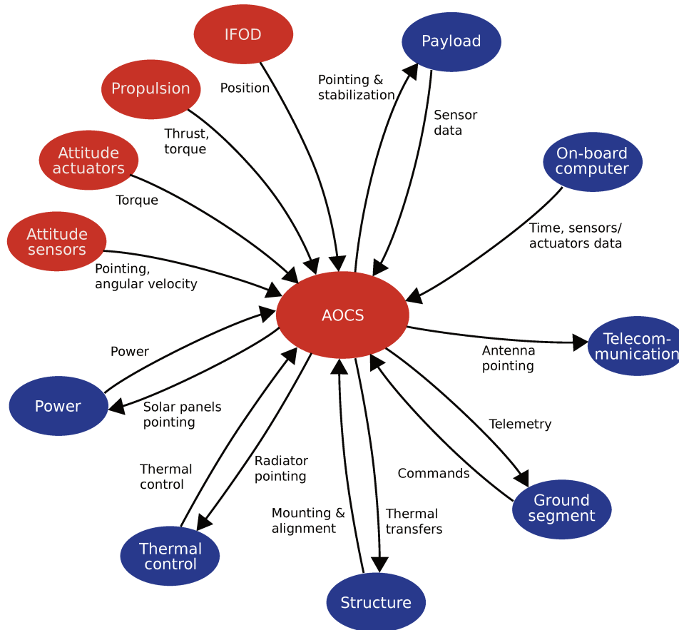
Figure III.4: Functional relationships between the Attitude & Orbit Control System (AOCS) and the other subsystems of a spacecraft. The AOCS is decomposed into its main components in red, while other subsystems are in blue.
