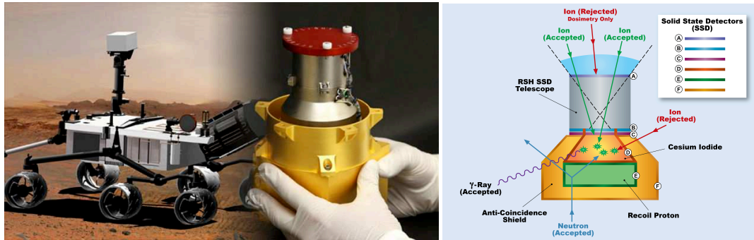
Figure I.4: MSL-Curiosity rover and its Radiation Assessment Detector (RAD) instrument (left). Schematic of the working principle of RAD (right). Credit: NASA and Southwest Research Institute.
