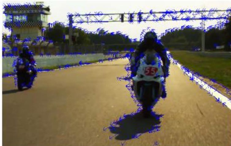
Figure 7: Velocity vectors of some points of interest in a frame computed by the Lukas Kanade OF approach
