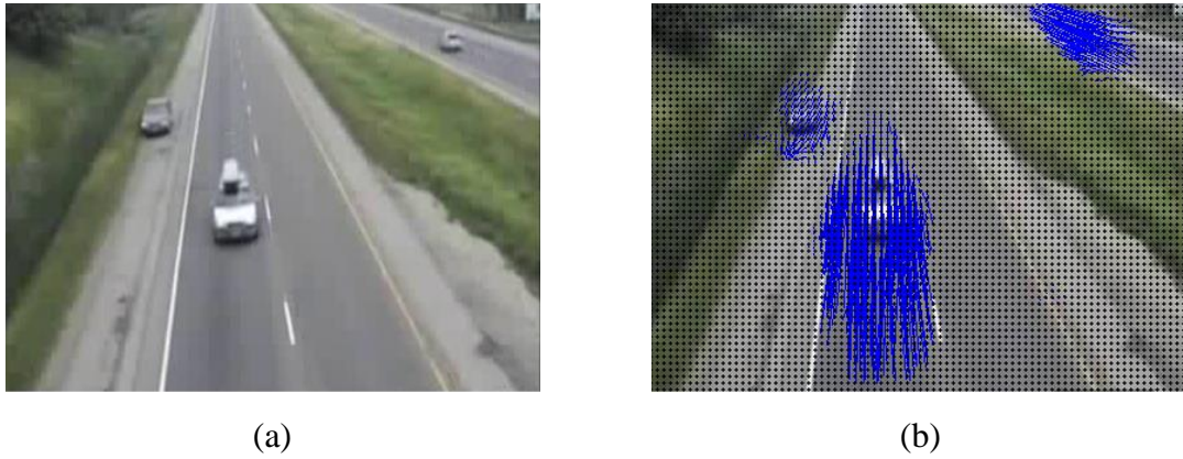
Figure 8: The results of Farneback OF applied on a traffic scene. (a): the original frame, (b): the drawing in blue of the velocity vectors computed with the Farneback OF.
