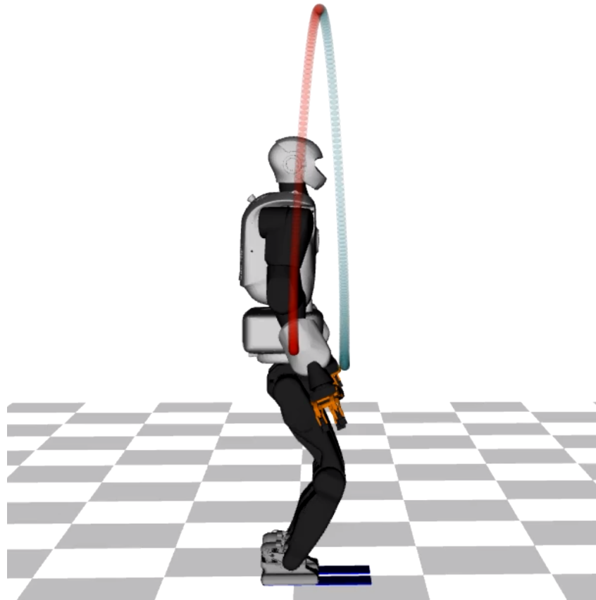
Fig. 6.2: Solution of the Centroidal Optimization Problem (6.1). The ball shows the trajectory followed by the center of mass, when we obtain the solution of our optimization problem (6.1). Since we did not consider the feasibility constraints, the solution assumes really long robot legs. This trajectory can be improved by taking kinematic information in our optimization.
