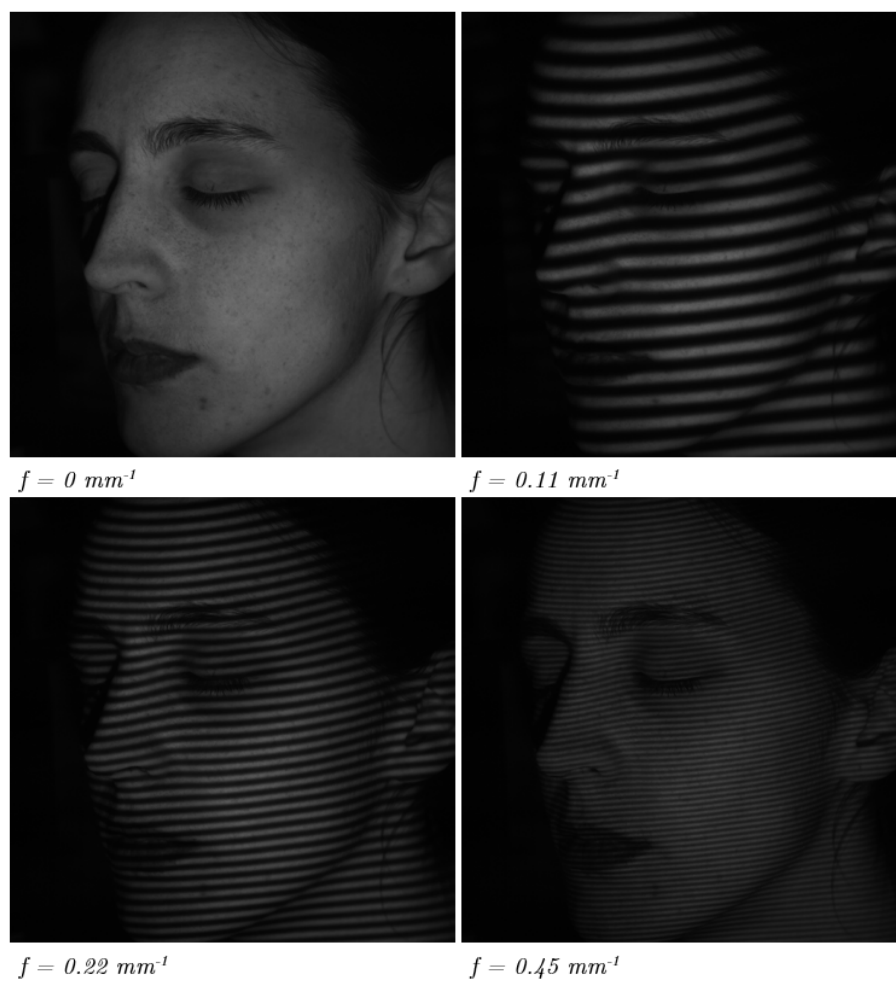
Figure 8.11. SFDI acquisition at four frequencies on a full face, side view acquisition.
