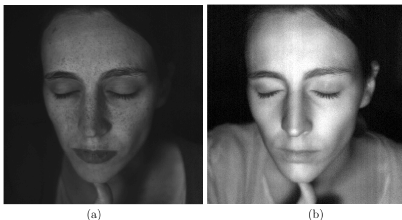
Figure 4.4. Full face hyperspectral acquisition using the SPECIM IQ camera (Specim, Finland), image displayed at (a) 446 nm and (b) 785 nm.
