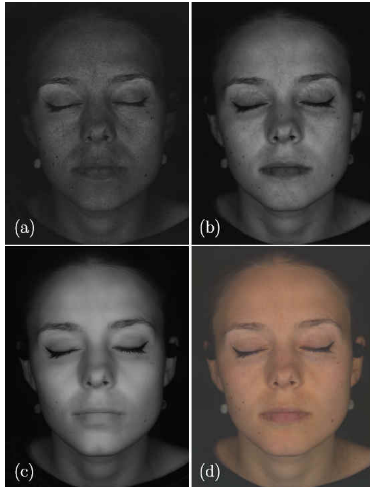
Figure 4.18. Example of channels of a hyperspectral image of a face: Image (a) at 420 nm, (b) at 590 nm, (c) at 700 nm, and (d) color image after conversion into RGB values. (These images can be found in large format in Appendix 1).
