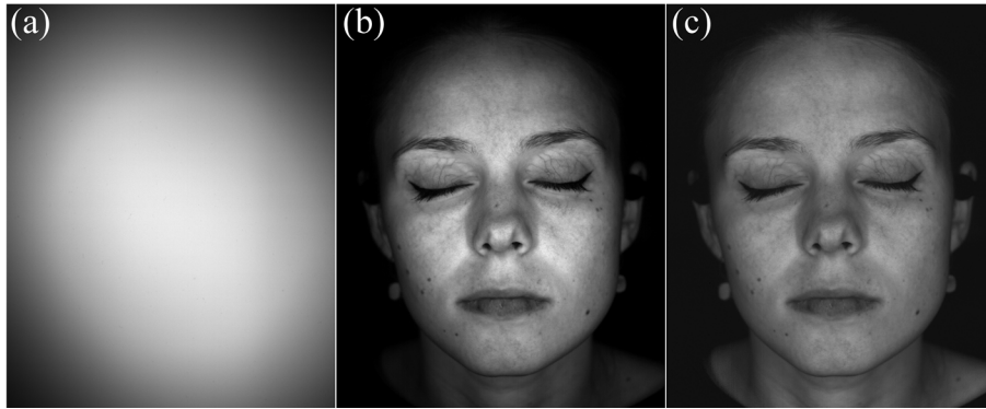
Figure 4.14. Acquired and corrected images at 590 nm: (a) Non-uniform illumination on the white reference plane, (b) uncalibrated image, (c) calibrated image.
