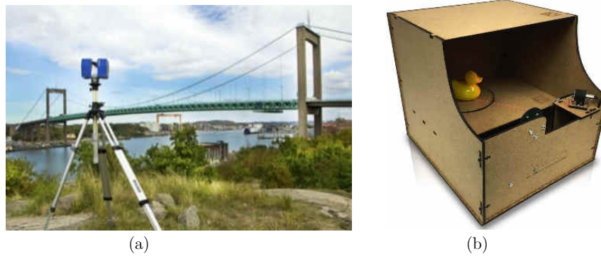
Figure 5.4. (a) 3D laser scanner (FARO, USA), (b) FabScan Pi slit scanner (Open source kit [Herakleous and Poullis]).
