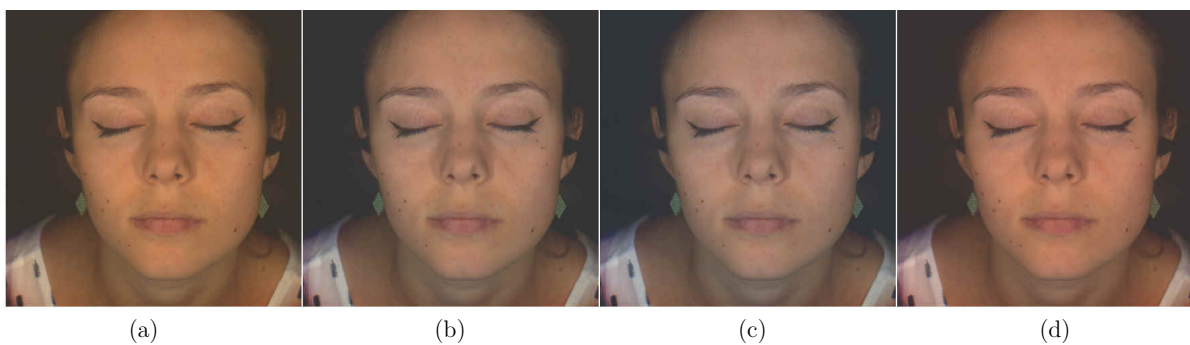
Figure 4.19. Color image under several illuminants: (a) D50, (b) D65, (c) D75 and (d) E illuminant.
