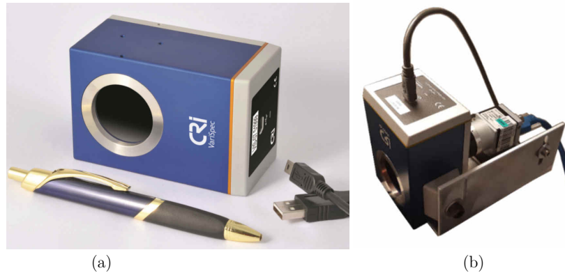
Figure 4.3. (a) VariSpec™ LCTF (PerkinElmer, USA), (b) LCTF mounted in front of a monochromatic camera.
