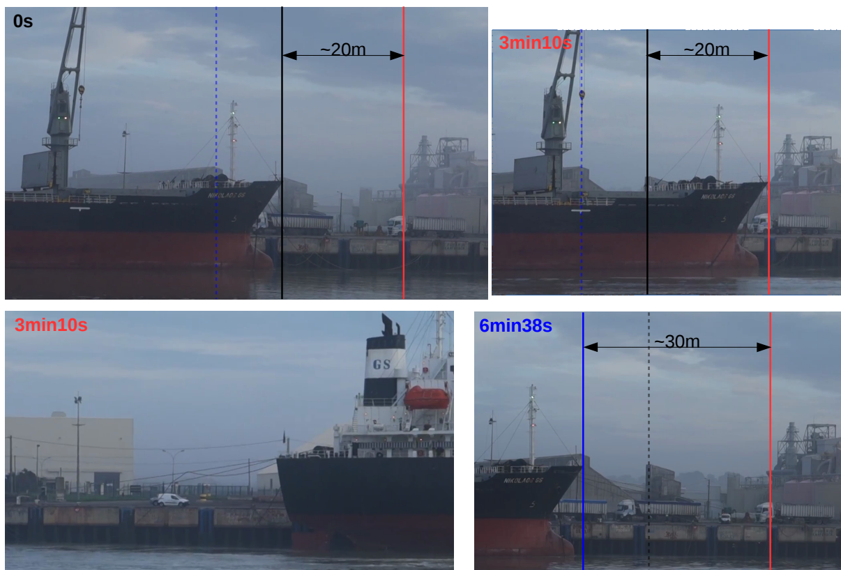
Figure 2.10 – Snapshots presenting the amplitude of moored boat surge motion. The lower pictures show the excessive tensions in the mooring lines, on the right picture (6min38s) a line was broken. Distances are estimated based on the 12 m gap between the docking fenders. Photos by Denis Morichon, reproduced with permission.
