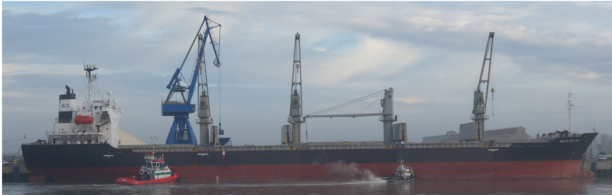
Figure 2.9 – Surge motion of the moored bulk carrier Nikolaos GS, February 16, 2018 at 9am (UTC+1). To limit the movement amplitude, two tugs pushed the vessel against the wharf on docking fenders. The cargo was moored at Tarnos terminal with the bow facing upstream. The view was taken from the marina. Photo by Denis Morichon, reproduced with permission.
