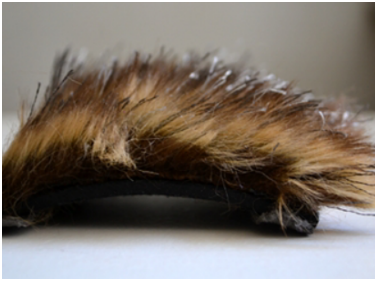
Figure 3.21: Conductive fur, conductive yarns are mixed within the fur.
