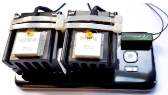
Figure 3.12: Multi-Moji uses multi-modal cues (including tactile) to convey a wide range of emotions from a smartphone. [Wilson and Brewster, 2017]
