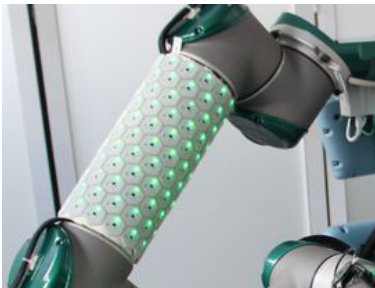
Figure 3.22: Spatially reconfigurable robotic cells that embed a variety of sensors: touch, temperature,..
