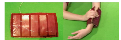
Figure 3.14: Interface that warp around the forearm, that uses pneumatic compression to compress the user.
