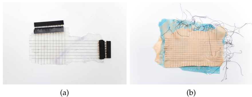
Figure 8.6: Tests of conductive yarns. a) The first interface was designed with non-stretchable conductive yarns. b) Another test on a larger surface with stretchable yarns
