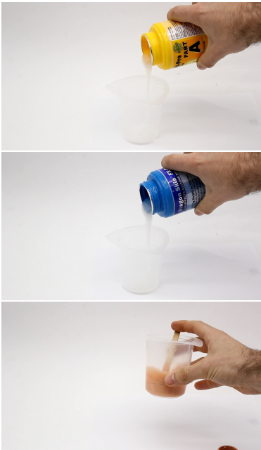
Figure 7.6: The three fabrication steps to prepare the silicone [Smooth-On, 2019b]. 1) Part-A of the silver cured silicone is poured onto the container. 2) An equivalent volume of Part-B Ecoflex silicone is poured. 3) Finally, the two parts are mixed thoroughly with silicone pigments.
