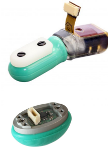
Figure 7.2: BioTac robot finger, with an extremely high sensing acuity that uses different viscosity to reproduce human's viscosity
