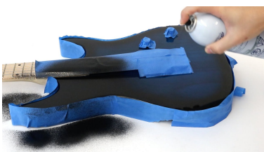
Figure 3.19: Covering existing objects with conductive paint enable detecting touch through EIT sensing.
