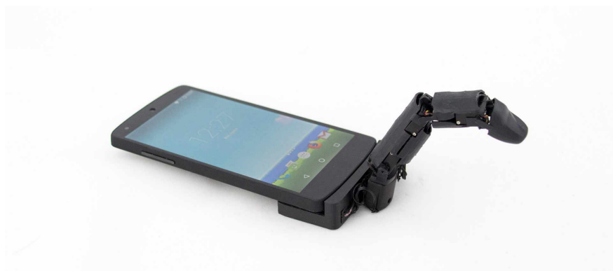
Figure 6.1: MobiLimb is a robotic interface is connected to a smartphone, and can provide haptic feedback to the user.
