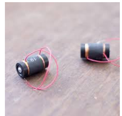
Figure 3.3: Haptuators vibration motors, capable to perform a wide range of vibration frequencies.
