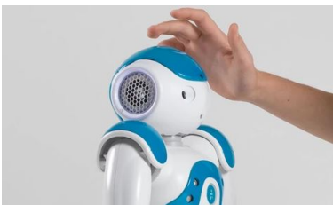
Figure 4.13: Nao Robot being touched on the head, where a touch sensor is located.
