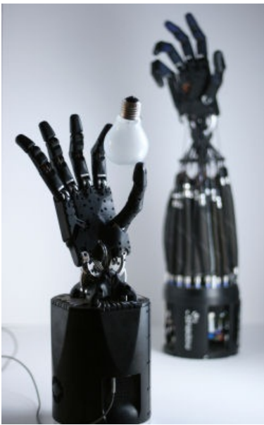
Figure 4.12: The Shadow Hand by Shadow Robotics, a hand with five fingers and a pneumatic muscle-like actuation
