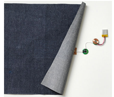
Figure 3.20: Project Jacquard , textile augmented with conductive yarn to detect capacitive touch.
