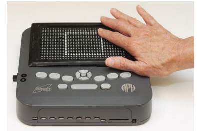
Figure 3.10: Braille cells capable to display figures and graphical elements [Vidal-Verdú and Hafez, 2007]
