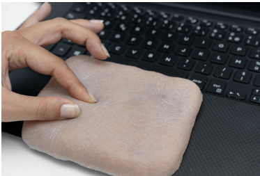
Figure 7.17: Closeup of the anthropomorphic skin-like touch-pad. We can see the details of the wrinkles.
