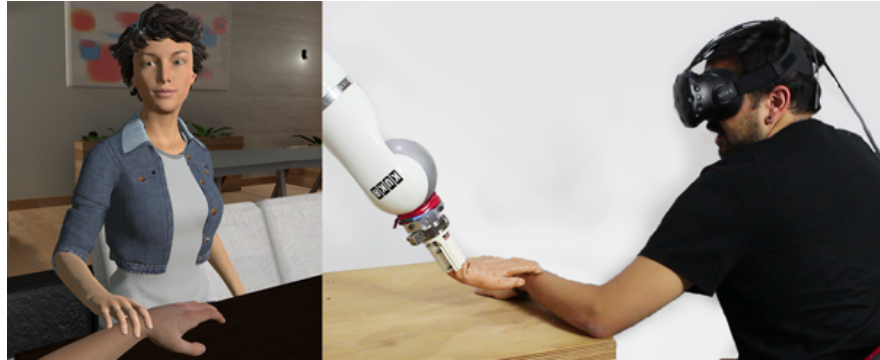
Figure 5.13: Combination of a VR visual (left) and Haptic (right) feedback to increase the communicative capabilities of a virtual agent.
