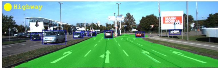
Figure 1.2: MultiNet real-time predictions for road-type classification, vehicle detection and road segmentation.
