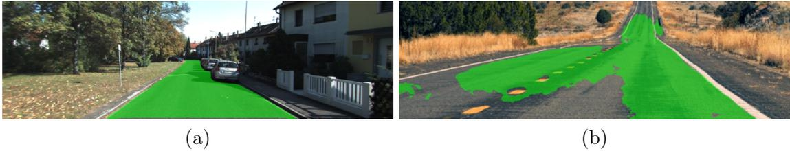
Figure 1.3: MultiNet overfitting issue for road segmentation task: A lack of generalization capacity when not trained on the target domain data. These images present MultiNet road segmentation pixel-level predictions on a Kitti dataset image (a) and on an image of a desert road (b).
