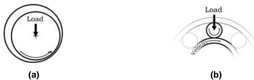
Figure I.3. Schematic representation of the geometries of: (a) a conformal contact in a journal bearing, and (b) a non-conforming contact in a roller bearing [79].
