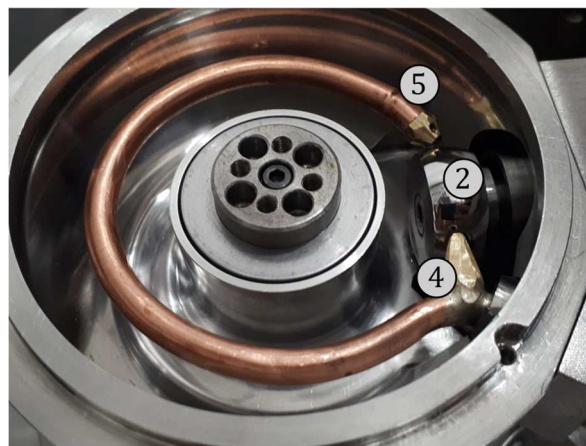
Figure 2.2-2 – Photo of the projection system (4) (5) and the mounted barrel (2). The disc is not mounted.
