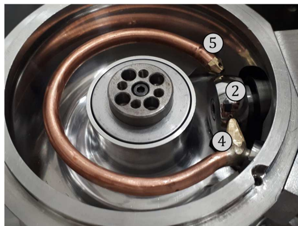
Figure 2.2-2 – Photo of the projection system (4) (5) and the mounted barrel (2). The disc is not mounted.
