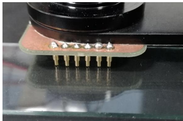
Figure 37: Conductivity measurement setup for soft substrates. The pins were large to avoid the substrate to be pierced.
