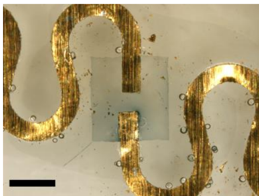
Figure 48: Zoom of the final device on the channel. In blue, the PEDOT, patterned by photolithography in a square shape. The size of the square is voluntarily very large compared to the channel size, to see more easily later the effect of the stretch on the PEDOT:PSS. Scale bar is 500 \mu m.
