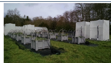
Figure 2: Experimental design used to answer questions i and ii. Plant roots and leaves are sampled at several times, corresponding to different development stages of oilseed rape. Question i requires to use cages when infesting plants by D. radicum while question ii does not in order to follow wild insect populations.
