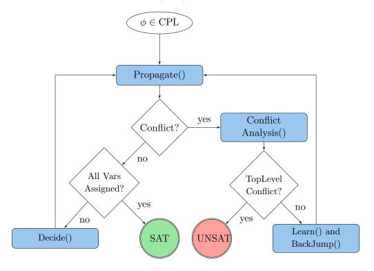
Figure 3.1: Schema of the CDCL Framework
