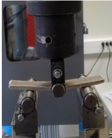
Figure 2.32. Essai cyclique de flexion 3-points
