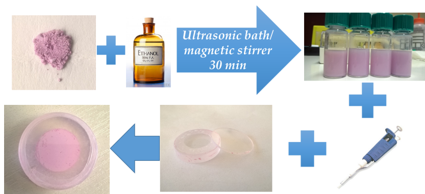
Figure 4.7 – [\text{Fe}(\text{NH}_2 - \text{trz})_3](\text{Br})_2 suspension preparation routine for shock experiment: 50 mg of nanoparticles are dispersed in 1 mL of ethanol and mixed in ultrasonic bath or magnetic stirrer for 30 min. Then a few drops of obtained liquid suspension are sandwiched between two glass substrates separated with a spacer.
