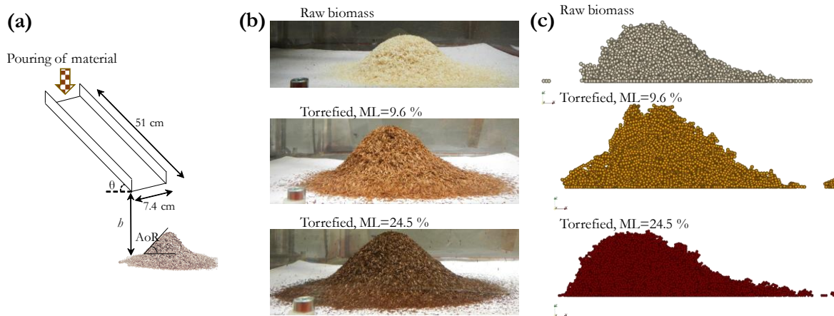
Figure 109. Calibration bulk experiment (Heap formation). (a) Main setup dimensions. (b) Examples of formed heaps for the biomass samples. (c) Corresponding DEM simulations.
