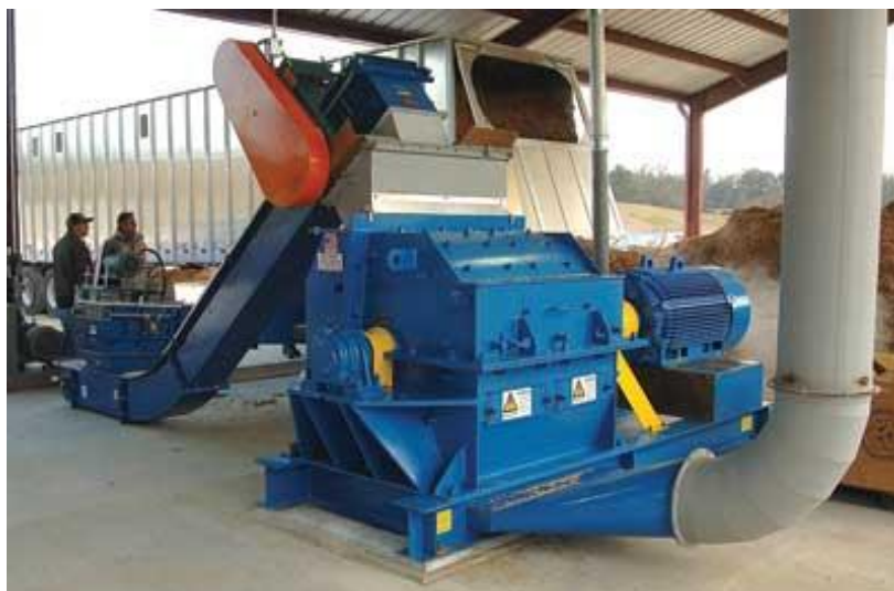
Figure 14. Hammer mill grinding woody biomass [86].
