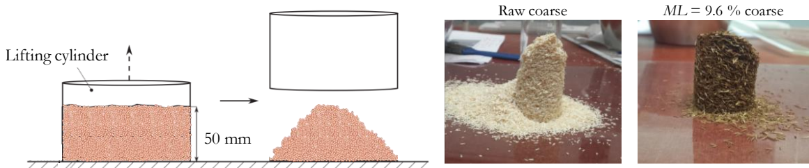
Figure 98. Lifting cylinder preliminary tests. (a) Schematic of the experiment (adapted from [380]). (b) Examples of the stable stacks of biomass formed.
