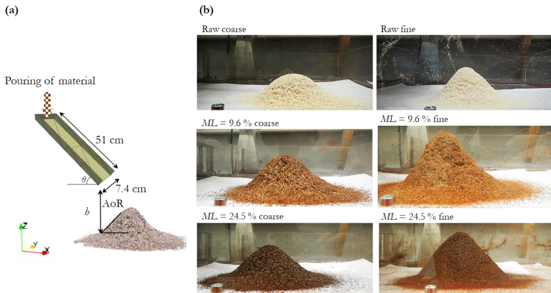
Figure 99. Angle-of-repose experiments. (a) Schematic representation of the main setup and dimensions. (b) Examples of the heaps formed for the biomass powders.
