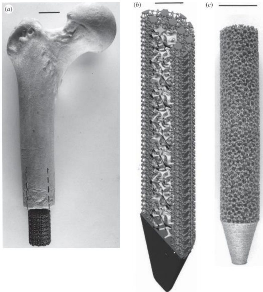
Figure 35: Illustration of multi-structural stem with dense ( 1.06 \text{ g.cm}^{-3} ) and less dense ( 0.58 \text{ g.cm}^{-3} ) areas for femoral implantation. The CAD (b) and EBM-built prototype (c) were derived from femoral model (a). Scale bars of (a), (c) = 2 cm and (b) = 1 cm from 85
