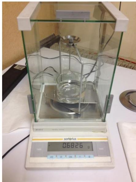
**Figure 69:** Weighting scale equipped with a hydrostatic weight platform
