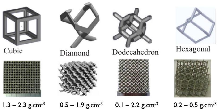
**Figure 34: Unit cells and corresponding lattices built by EBM with Ti-6Al-4V alloy.** Obtained lattices densities are close to human bone average densities which range from 0.19 to 1.99 g.cm<sup>-3</sup> (adapted from<sup>68</sup>)
