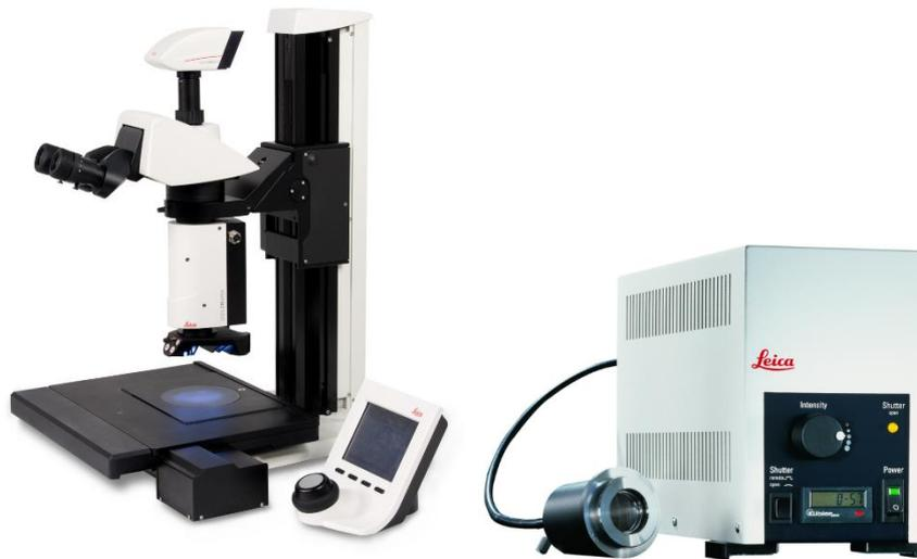
**Figure 81:** Illustration of the macro microscope Leica Z16 and the external mercury halide lamp. The fluorescence macroscopy system used was the combination of the macro microscope and the external lamp with a CCD digital camera (not represented here)<sup>183</sup>
