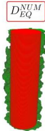
**Figure 101: Concept of mechanical equivalent diameter of EBM built struts.** The effective material involved in the mechanical response of EBM struts (represented by an equivalent cylinder of diameter  $D_{EQ}^{NUM}$ ) is lower than the total volume of the EBM built material (adapted from Suard<sup>175</sup>)
