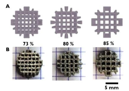
*Figure 98: CAD* (*A*) *and EBM built* (*B*) *Ti-6AI-4V architectured scaffolds with the expected porosities of 73%, 80% and 85%.* Respectively corresponding to 7, 6 and 5 repeated unit-cells along the scaffold diameter
