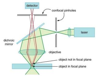
*Figure 83: Schematic representation of the confocal microscopy principle. Pinholes are specifically placed after the laser source and before the detector on conjugate planes to the focal plan observed on the probed sample to increase the images resolution*<sup>185</sup>
