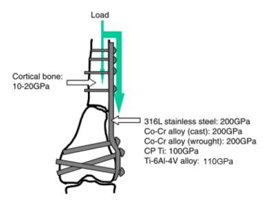
Figure 29: Illustration of the load distribution in presence of metallic bone fixation which can induce a stress shielding effect. Elastic modulus of cortical bone and the possible different material that can be used as metallic fixation are listed in  $GPa^{69}$
