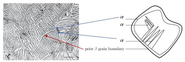
**Figure 65:** Micrograph (right) and schematic representation (left) of the typical microstructure of Ti-6Al-4V obtained by EBM, exhibiting the  $\alpha$  (hexagonal) + 6 (cubic) microstructure (scale bar = 50  $\mu$ m, from<sup>85,166</sup>)
