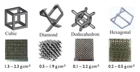
*Figure 34: Unit cells and corresponding lattices built by EBM with Ti-6Al-4V alloy.* Obtained lattices densities are close to human bone average densities which range from 0.19 to 1.99 g.cm<sup>-3</sup> (adapted from<sup>68</sup>)
