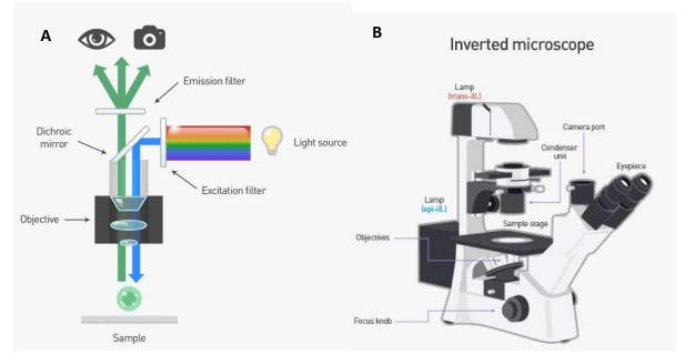
*Figure 82: Schematic presentation of the principle of epifluorescence microscopy* (*A*) *and the associated inverted fluorescence microscope* (*B*). The source light crosses the dichroic mirror and the objective to illuminate the sample. The light emitted by the sample passes through the same objective and mirror until reaching the emission filter<sup>184</sup>
