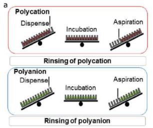
Figure 75: Schematic of layer-by-layer film deposit using the automated liquid handling machine into 96 well plates<sup>179</sup>
