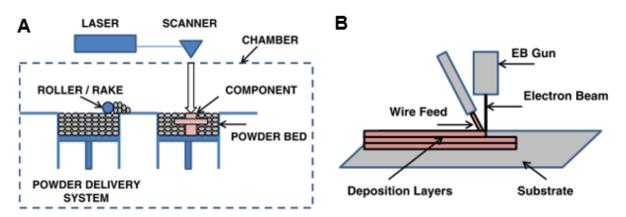
*Figure 32: Schematic representation of powder bed fusion* (*A*) *and wire based* (*B*) *additive manufacturing systems.* In powder bed fusion systems, the starting material is a powder that is deposited on the build platform for further melting. In wire based systems, the starting material is a wire directly deposited and melted after deposition<sup>80</sup>
