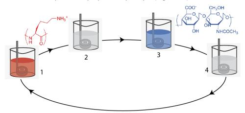
Figure 77: Schematic representation of the automated dipping method for the PEM film deposition into 3D architectured scaffolds
