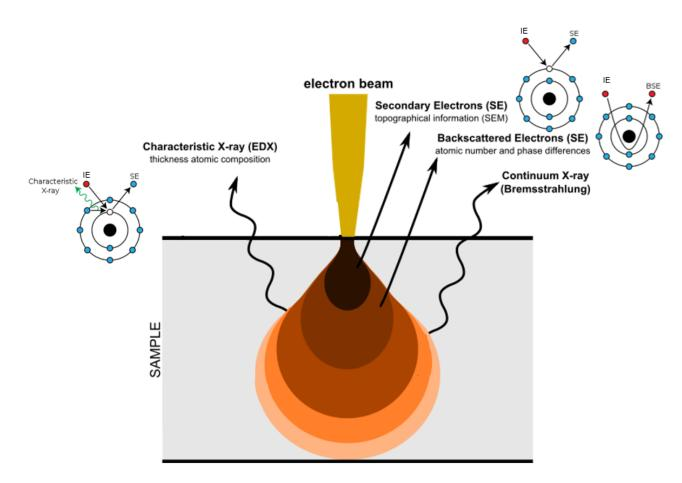
*Figure 84: The different physical phenomena resulting from the electron/matter interaction detected by the scanning electron microscope. Secondary, backscattered electrons and characteristic X-rays are detected to image and analyse the sample composition*<sup>187</sup>
