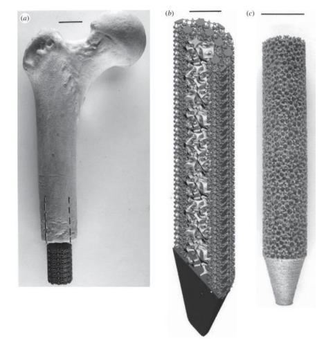
Figure 35: Illustration of multi-structural stem with dense (1.06 g.cm<sup>-3</sup>) and less dense (0.58 g.cm<sup>-3</sup>) areas for femoral implantation. The CAD (b) and EBM-built prototype (c) were derived from femoral model (a). Scale bars of (a), (c) = 2 cm and (b) = 1 cm from<sup>85</sup>
