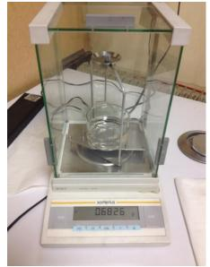
Figure 69: Weighting scale equipped with a hydrostatic weight platform
