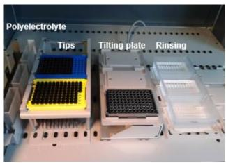
*Figure 74: Working table of the automated liquid handling machine used for the film deposition in cell culture well plates.* The polyelectrolyte solutions are in reservoirs, the tips on tip holders while the well plates are placed on a tilting plate carrier. The reservoir containing the rinsing solutions are placed on the right side of the working table.
