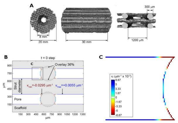
Figure 37: Representation of mPCL-6-TCP scaffolds with 0/90° strut laydown pattern (A) and the corresponding mean surface curvature estimations (B) and zoom (C) in a unit volume of those scaffolds ( $adapted from^{93}$ )
