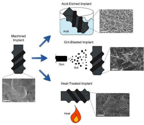
Figure 42: Schematic representation and corresponding SEM images of three main surface modification techniques applied to titanium implants to increase the surface roughness: acidetching, grit-blasting, heat-treatment. Scale bar =  $3 \mu m$  from<sup>105</sup>
