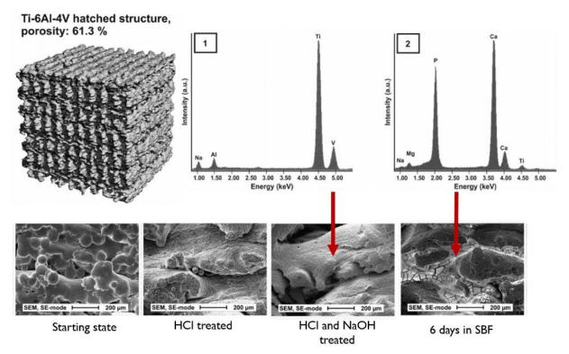
**Figure 43: Representation of the EBM built Ti-6AI-4V hatched lattice.** Scanning electron microscopy images of non-treated, acid treated (HCl), acid and alkali treated (NaOH) and simulated body fluid treated (SBF) surfaces and the corresponding EDX analysis for HCl/NaOH treated (1) and SBF treated (2) surface (adapted from<sup>106</sup>)
