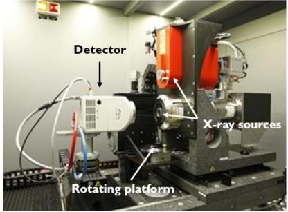
Figure 71: Internal view of the EASYTOM XL tomograph (adapted from<sup>174</sup>)
