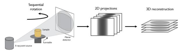
*Figure 70: Principle of the X-ray tomography imaging technique* (adapted from<sup>172</sup>)
