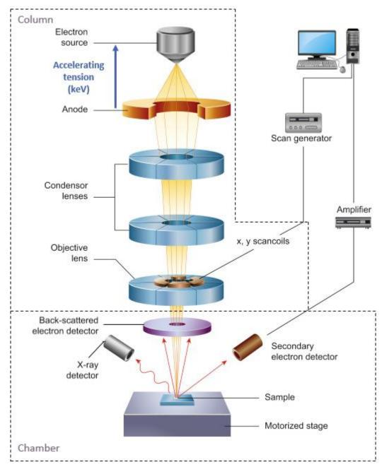
*Figure 85: Scheme of the scanning electron microscope.* The scanning electron beam is generated and controlled in the column, the emitted signals from the electrons/matter interaction are detected in the chamber (adapted from<sup>188</sup>)
