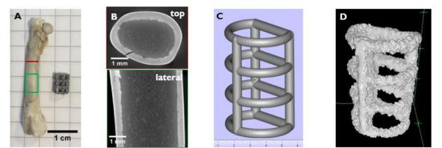
**Figure 117: Design strategy for in vivo experiments using an architectured Ti-6AI-4V implant adapted for a critical size femoral bone defects in rat.** (A) Representation of the rat femur and one of the EBM built Ti-6AI-4V implant for implantation (B) Cross and lateral sections of the rat femur obtained by Xray tomography prior implantation (C) Computed Aided Design of one of the Ti-6AI-4V implant (D) 3D representation of EBM built Ti-6AI-4V implant obtained by X-ray tomography
