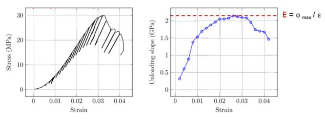
*Figure 73: Example of the stress-strain cycles applied to architectured Ti-6AI-4V scaffolds* (*left panel*) *and the corresponding representation of the unloading elastic modulus versus strain* (*right panel*). *The global elastic modulus was determined as the maximum value of the curve (adapted from* <sup>166</sup>)
