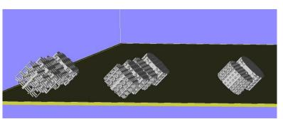
*Figure 68: Representation of the scaffolds placement into the build platform with a 45° angle*
