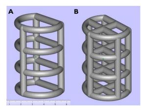
**Figure 118: CAD representation of in vivo Ti-6AI-4V implants for critical size femoral bone defect in rat.** The two type of implants with a 1 cm<sup>2</sup> (A) and 1.5 cm<sup>2</sup> (B) total surface areas are respectively represented
