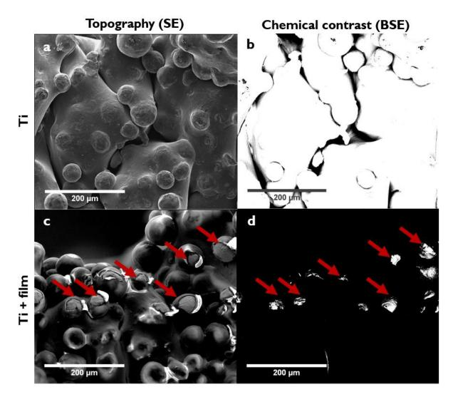
**Figure 112: Coating of architectured Ti-6AI-4V scaffolds with (PLL/HA)**<sub>24</sub> **PEM film.** Ti-6AI-4V architectured scaffolds bare and coated with (PLL/HA)<sub>24</sub> observed under scanning electron microscopy (SEM) in topography mode (secondary electrons, a and c panels) and chemical contrast mode (backscattered electrons, b and d panels). The red arrows show scratched and uncovered areas of the scaffold surface
