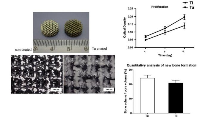
Figure 45: Picture of non-coated and Ta-coated EBM-built Ti-6AI-4V scaffolds and their respective surface microscopic images (left panels). Control of the mesenchymal stem cells proliferation on bare and Ta-coated scaffolds after 1, 4 and 7 days (right). Quantitative analysis of the bone formation on Ta-coated and bare scaffolds 12 weeks post-implantation in goat iliac crests (adapted from<sup>109</sup>)
