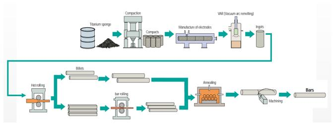
*Figure 30: Manufacturing processes to obtain Titanium bar stocks. Titanium sponge are mixed with alloying elements and prepared as electrodes for their melting. The obtained ingot is further processed with hot rolling and annealing steps to obtain titanium bars (adapted from*<sup>74</sup>)
