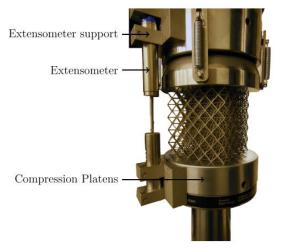
Figure 72: Compression device used to perform mechanical tests on architectured scaffolds<sup>166</sup>
