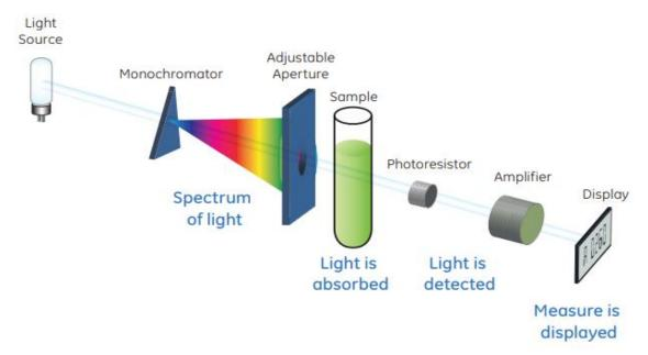
*Figure 79: General principle and components of a spectrophotometer.* The light is produced by a source light and travels through the monochromator and an adjustable aperture to illuminate the sample. The transmitted light is detected through a photoresistor<sup>181</sup>
