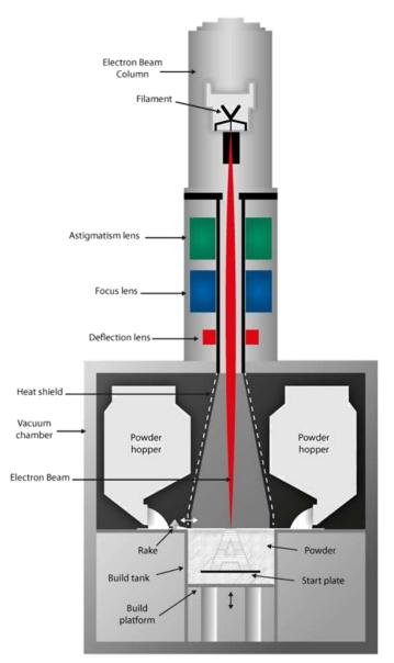
*Figure 67: Schematic presentation of the EBM machine.* The upper part is the electron beam column and the bottom part represents the build chamber<sup>168</sup>
