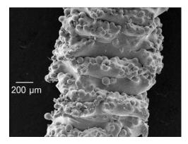
*Figure 99: Rough surface of Ti-6Al-4V scaffolds built by EBM.* The image was acquired by scanning electron microscopy<sup>166</sup>
