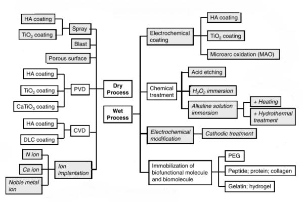
Figure 41: Overview of the existing surface treatment processes used for metallic bone substitutes at the research and clinical stages<sup>69</sup>
