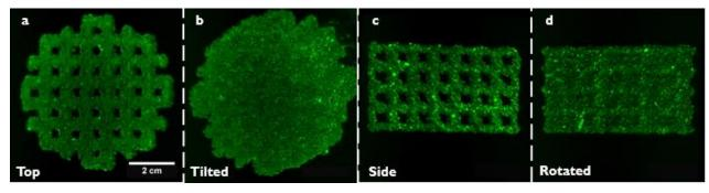
**Figure 111: Coating of architectured Ti-6AI-4V scaffolds with (PLL/HA)**<sub>24</sub> **PEM film.** Ti-6AI-4V architectured scaffolds coated with (PLL/HA) <sub>24</sub> + (PLL-<sup>FITC</sup>/HA) observed by fluorescence macroscopy with (a) top view, (b) tilted, (c) lateral view, (d) rotated
