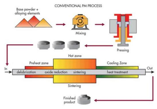
*Figure 31: Representation of powder metallurgy manufacturing process.* Powders are mixed and pressed into a designed mould. Moulds are heated to sinter powders before obtaining the finished product<sup>79</sup>
