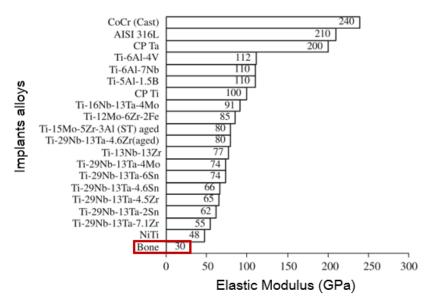
Figure 28: Elastic modulus of alloys used for bone implant<sup>67</sup>
