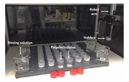
*Figure 76: Picture of the automated dipping robot DR3 for the film deposition on 3D architectured scaffolds.* The polyelectrolytes and rinsing solutions are in beakers, where the robot arm is successively dipped into following a custom-made procedure. The total duration for the deposition of 12 layer pairs is about 8 h.
