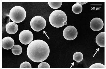
*Figure 66: Gas-atomized Ti-6Al-4V powder visualized under scanning electron microscopy*. The white arrows represent the necks from previous building uses<sup>166</sup>
