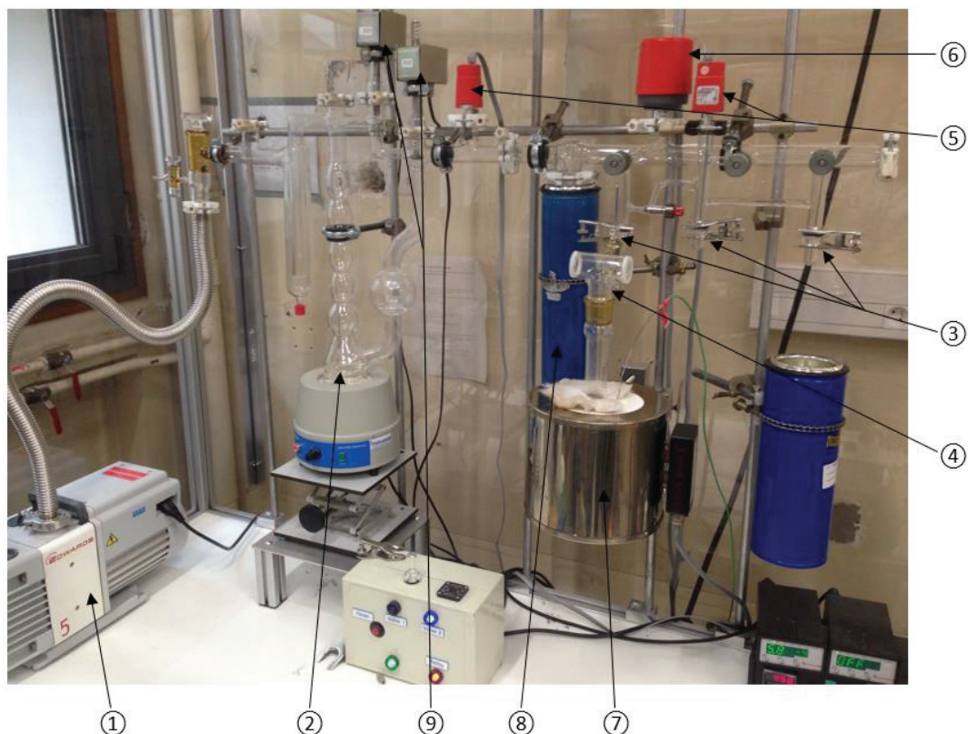
Figure 6. Picture of the vacuum ramp built for the characterization of acidity by use of pyridine as a probe molecule. Legend: ① Rotatory pump; ② Oil diffusion pump; ③ Rotulex™ connections; ④ IR sample cell; ⑤ Pirani gauges; ⑥ Active inverted magnetron gauge; ⑦ Furnace; ⑧ Liquid nitrogen trap; ⑨ Electrovalves security system.
