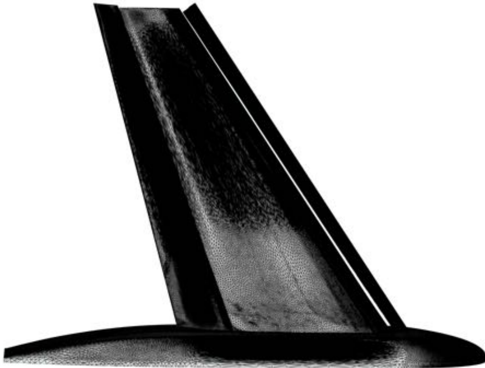
Figure 6.28: Trap wing: Top view of the 1.6 M nodes adapted surface mesh generated by the viscous adjoint-based adaptation on the lift.
