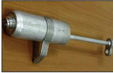
Figure 1.33: MPW application for automotive A/C receiver-dryer [62]
