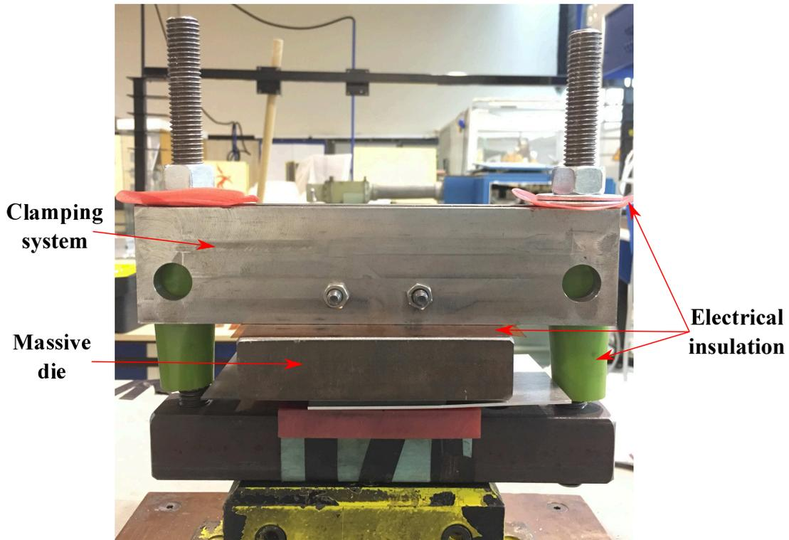
Figure 2.23: assembled mounting system in the O-shape coil case
