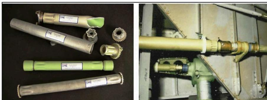
Figure 1.36: MPW application for aircraft flight control tubes [241]
