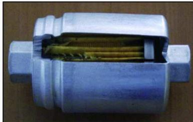
Figure 1.34: MPW application for fuel filter [62]
