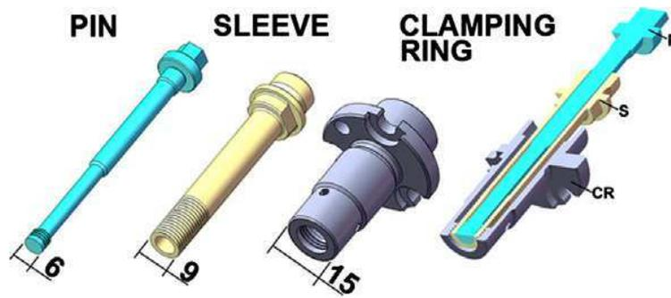
Figure 1.23: FSpJ tool system [72]
