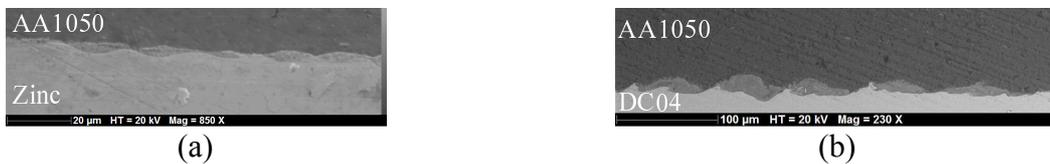
Figure 3.63: welding interface for (a) 1050 and pure zinc sheet; (b) 1050 and DC04
