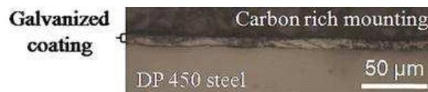
Figure 3.65: transverse cross section of the galvanized DP450 steel (light microscopy) [16]
