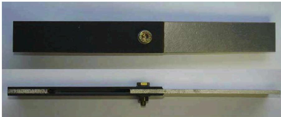
Figure 1.12: bonded/bolted hybrid joint CFRP/Al 7075-T62 [118]
