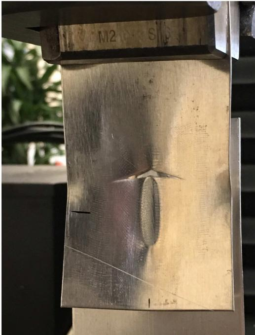
Figure 3.17: 5754 sheet teared during quasi-static lap shear test
