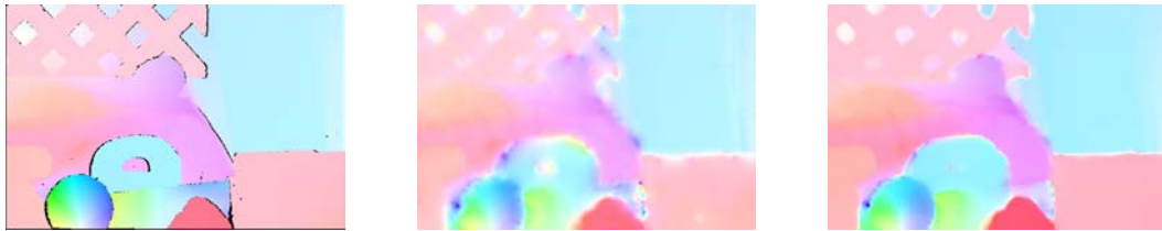
FIGURE 2.2 – 2D optical flow for a pair of images displayed using Middlebury style color coding. Left : ground-truth, Middle : Horn-and-Schunck method, Right : Brox's method.
