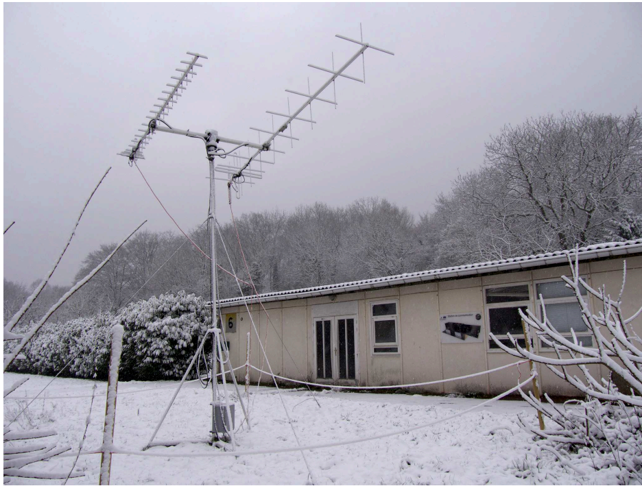
Figure 8.5: The ground station in Meudon, by a cold winter day. The antenna on the right is the emitting antenna, operating at 145 MHz, and the antenna on the left is the receiving antenna, operating at 435 Mhz.
