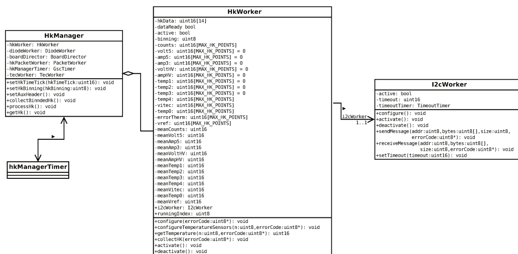
Figure 5.7: Class diagram showing the organization of the different software objects involved in house-keeping activities
