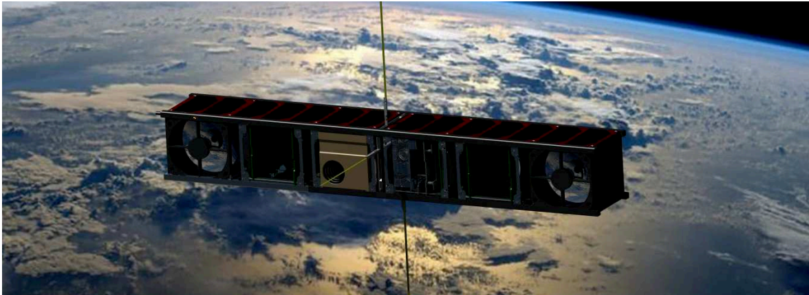
(a) SpaceFirst: a 6U nulling interferometer
