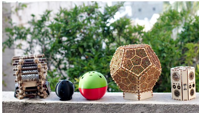
Figure 7.13: Various iterations were necessary in order to find a material which would be pleasing to hold (wood vs plastic), a structure that lets enough air flow toward the particles, and a shape which would create harmonious sound when the latter are fluttering (faces vs curves).
