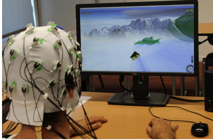
Figure 3.3: Participant using MI commands to play TuxRacer, e.g. imagining right hand movement to catch fish on the right.
