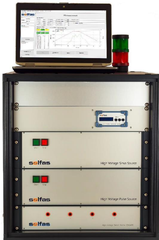
Figure 2.33. Partial discharges testbench by Solfas Technologie GmbH
