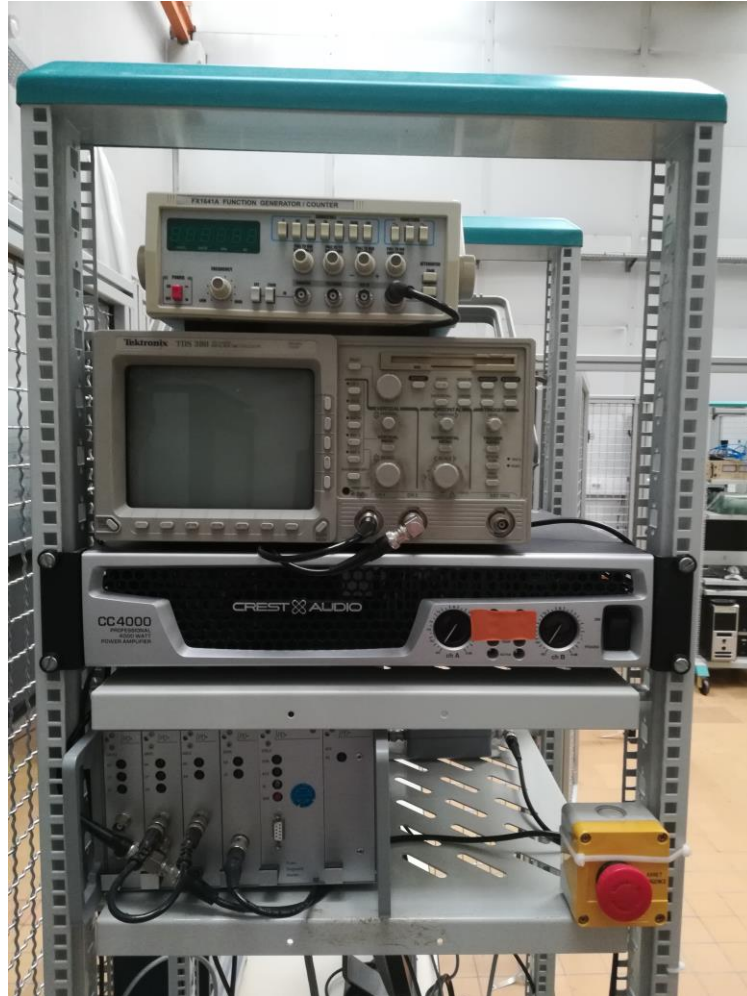
Figure 2.30. Partial discharges testbench by Power Diagnostix Systems GmbH
