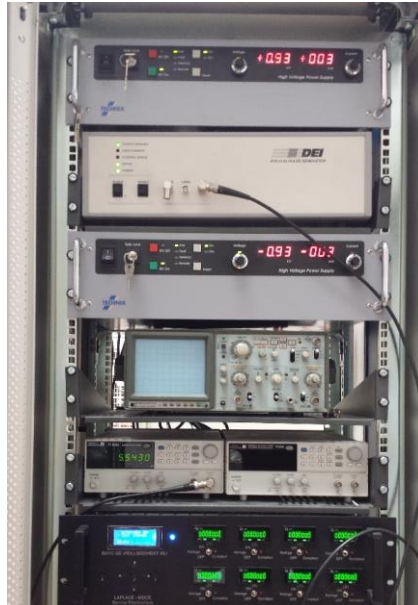
Figure 2.29. Rack with powering sources and lifespan counter for accelerated testbench
