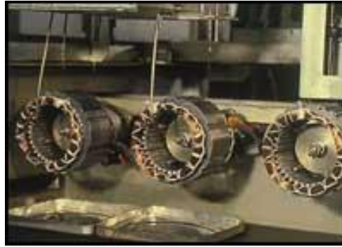
Figure 1.6. Trickle impregnation of a stator winding [8]
