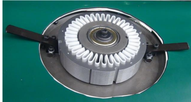
Figure 1.3. Stator core with slot liners in each slot [7]
