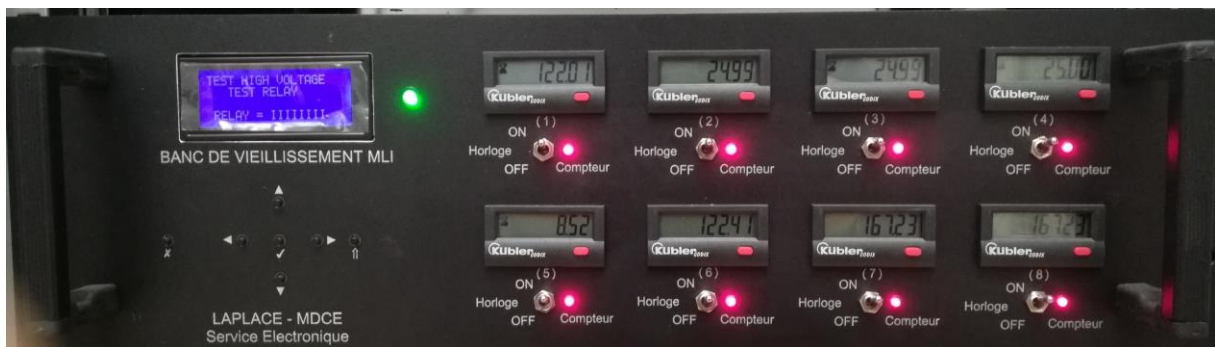
Figure 2.28. Test bench operating panel with 8 lifespan counters
