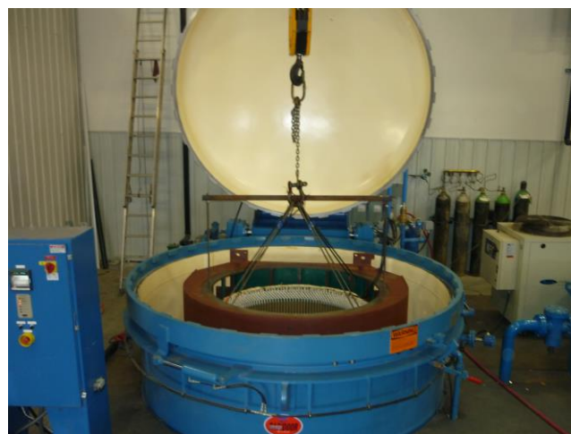
Figure 1.5. Tank used for Vacuum-Pressure Impregnation (VPI) [9]
