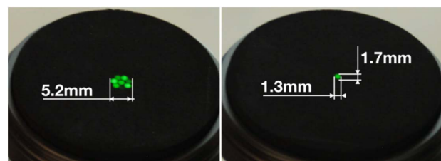
Fig. 4. Picture of the nominal illumination spot (left) and of the reduced illumination spot (right) of SHADOWS on a 2% Spectralon, seen from an emergence angle around 40^{\circ} .
