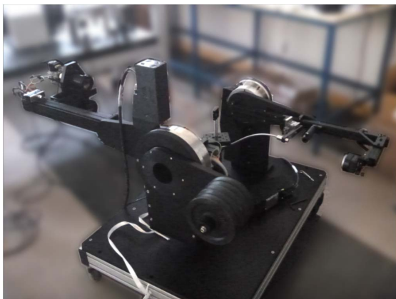
Fig. 6. SHADOWS goniometer in transmission mode. The sample is at the focal point of illumination.
