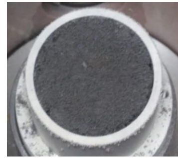
Sample before sublimation (diameter 5 cm, depth 5 mm)
