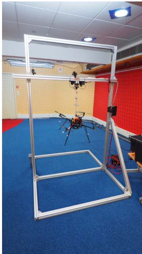
Figure 3.14 – Complete MonkeyRotor prototype with the structure for the branch.
