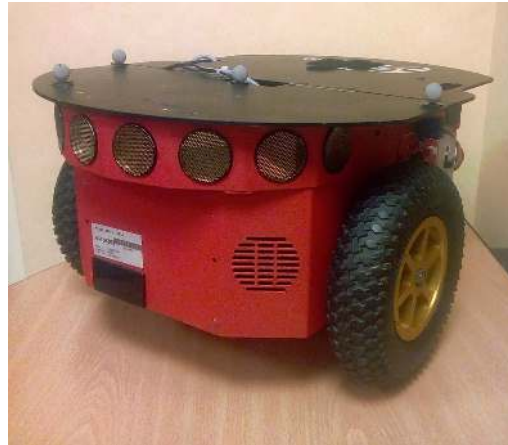
Figure 5.8 – The pioneer 3DX, a unicycle robot used for our experiments.
