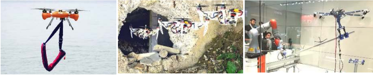
Figure 1 – Examples of modern applications of aerial robotics. On the left, a commercial product that is designed for waterproof rescue missions. On the middle, a foldable quadrotor able to adapt its shape from [23]. On the right, a cooperative framework sharing the task of moving an object between a grounded manipulator and an aerial robot, from [60].
