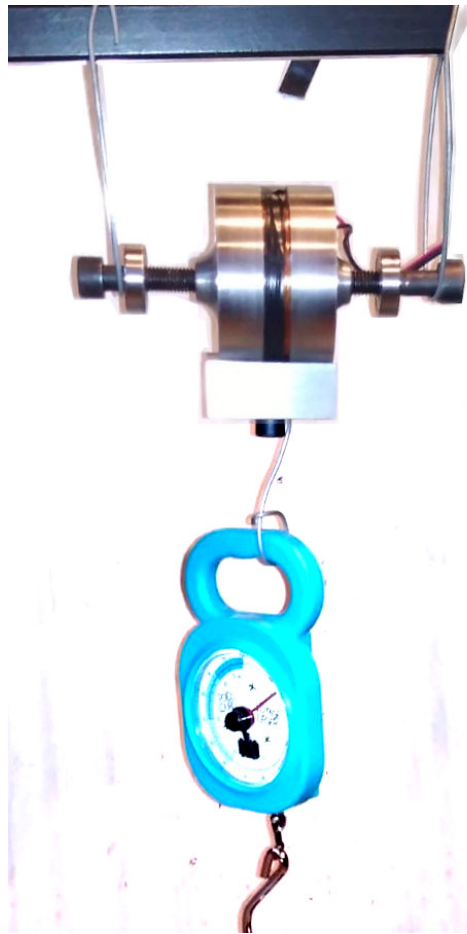
Figure 3.11 – Measure of the magnetic adhesion force with a dynamometer. The desired maximal load of 12 kg can be held as wished.
