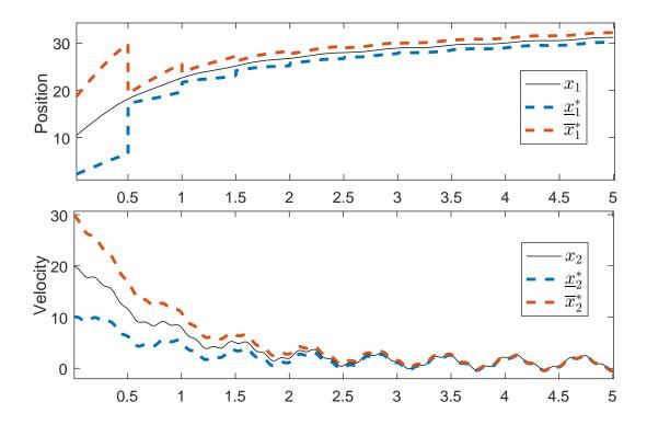
FIGURE 4.1: Simulation results for the UGV system: the attack-resilient estimate bounds for the position (top), and velocity (bottom).
