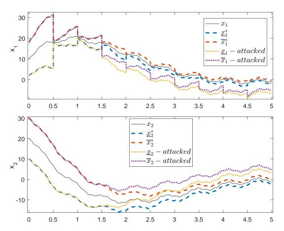
FIGURE 4.3: Simulation result for the academic system: the estimate bounds for the states  $x_1$  (top) and  $x_2$  (bottom), both attack-resilient estimate (dashed line) and attacked one (dotted line).
