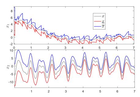
FIGURE 2.1: Simulation results for the spring-mass-damper system: the estimate bounds for the position (top), and velocity (bottom).
