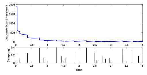
FIGURE 2.4: Simulation results: the Lyapunov function of the estimation error (top), the inter-measurement times (bottom).
