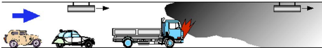
Figure 1.3: Fire-induced smoke longitudinal control [17].
