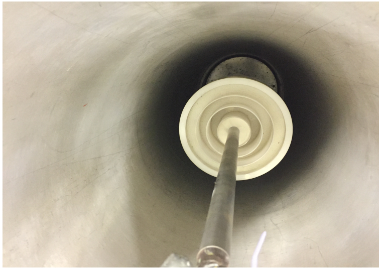
FIGURE B.6: Premixing phantom with its first ring filled with hafnia powder.
