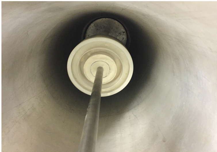
FIGURE B.7: Premixing phantom with its first and second ring filled with hafnia powder.
