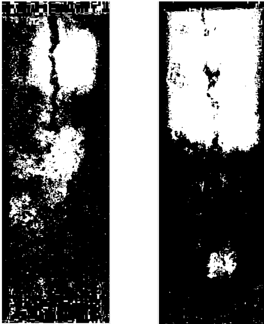
FIGURE 7.8: Otsu thresholding application; (left): image from the first premixing before explosion; (right): second premixing image after explosion .
