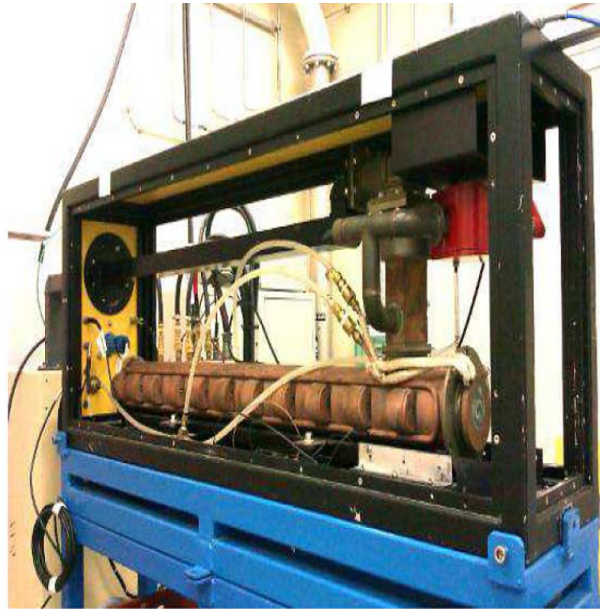
FIGURE 2.13: Linac Mini-Linatron Varian of KROTOS radioscopy system [40].
