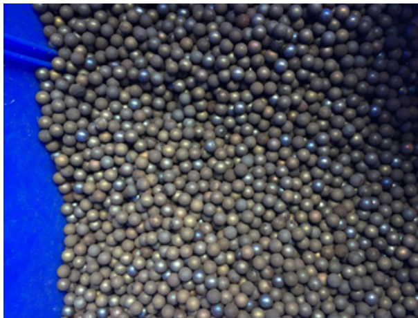
(a) Steel balls used in the experiment to represent corium fragments.
