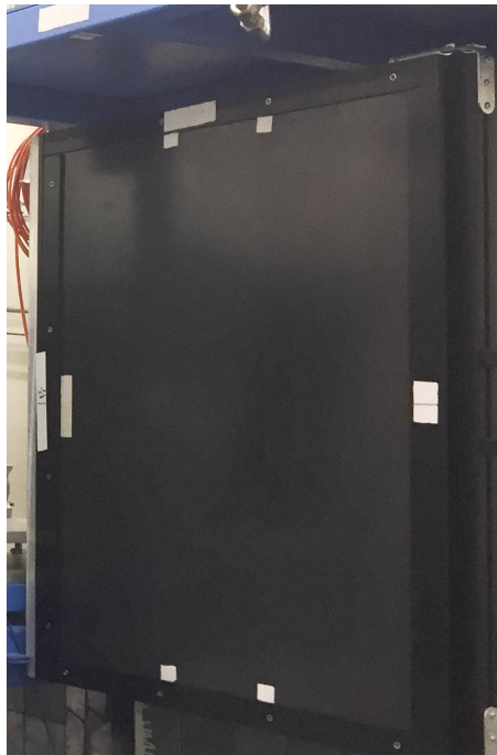
FIGURE 5.8: 2D scintillator detector at the KROTOS facility with a screen size 80 \times 60 \text{ cm}^2 [40].
