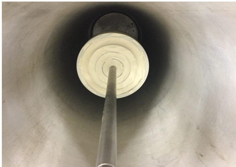
FIGURE B.9: Premixing phantom with its all 4 rings filled with hafnia powder.
