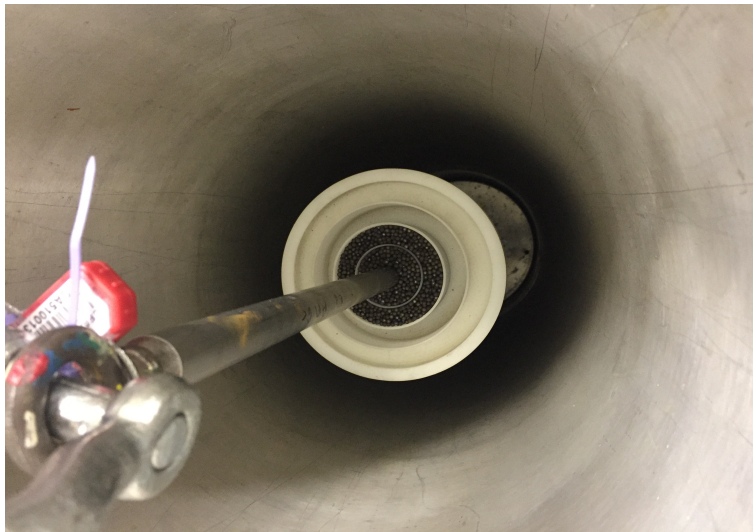
FIGURE B.3: Premixing phantom with its first and second ring filled with steel balls.
