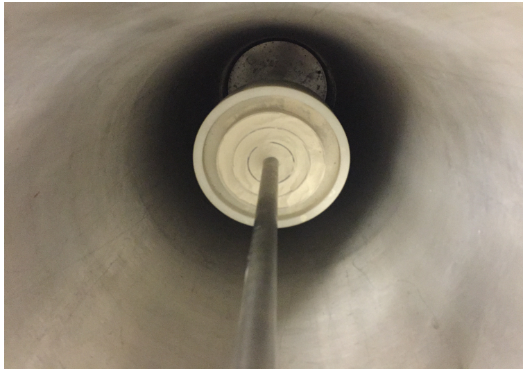
FIGURE B.8: Premixing phantom with its first three rings filled with hafnia powder.
