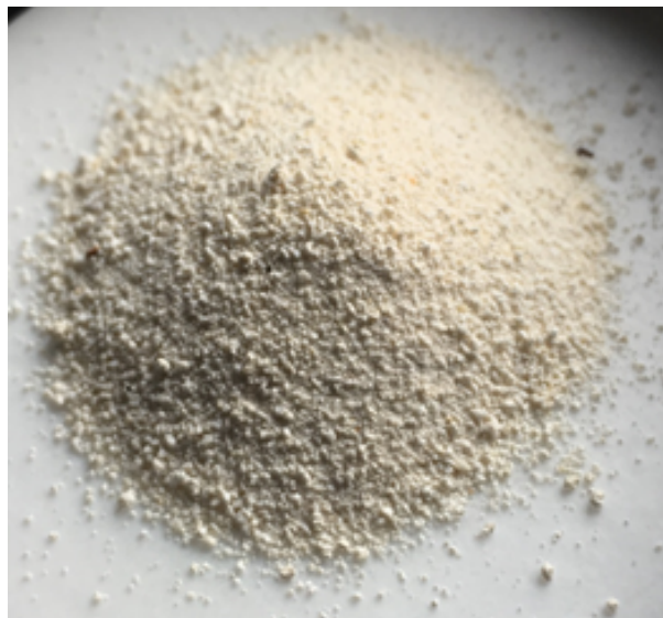
FIGURE 5.5: Hafnia powder representing less dense cloud of corium particles.
