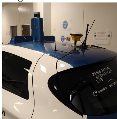
(b) Velodyne VLP32C and GNSS antenna
